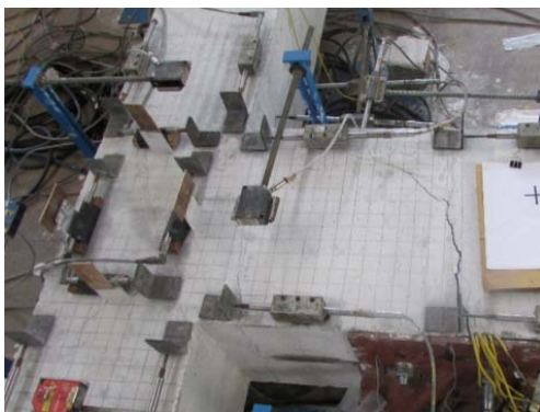
Fig. 9 Crack pattern observed at drift ratio of +1.47% for SP1-U1
