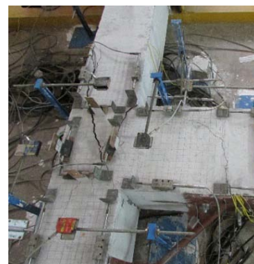
Fig. 11 Crack pattern of SP1-U1 at drift ratio of -2.94%
