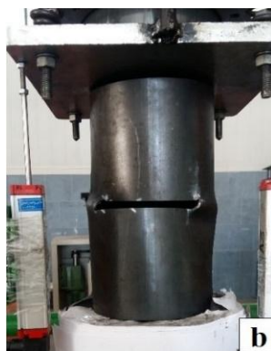
(b) Deformation of non-strengthened specimen
