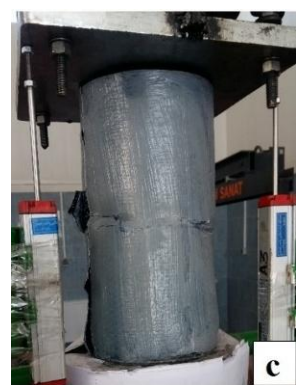
(c) Deformation of strengthened specimen by four CFRP layers
