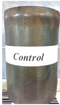
Fig. 12 Ultimate deformation of control (specimen without defect)
