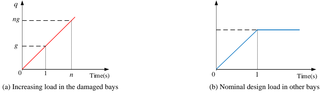
Fig. 18 Load applied curve in different bays
