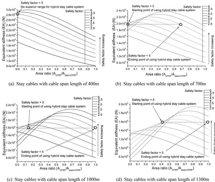
Fig. 7 Equivalent stiffness of stay cables with different cable span lengths
