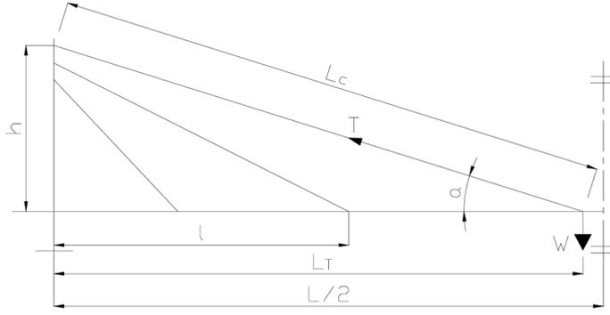
Fig. 1 Calculation model of stay cables
