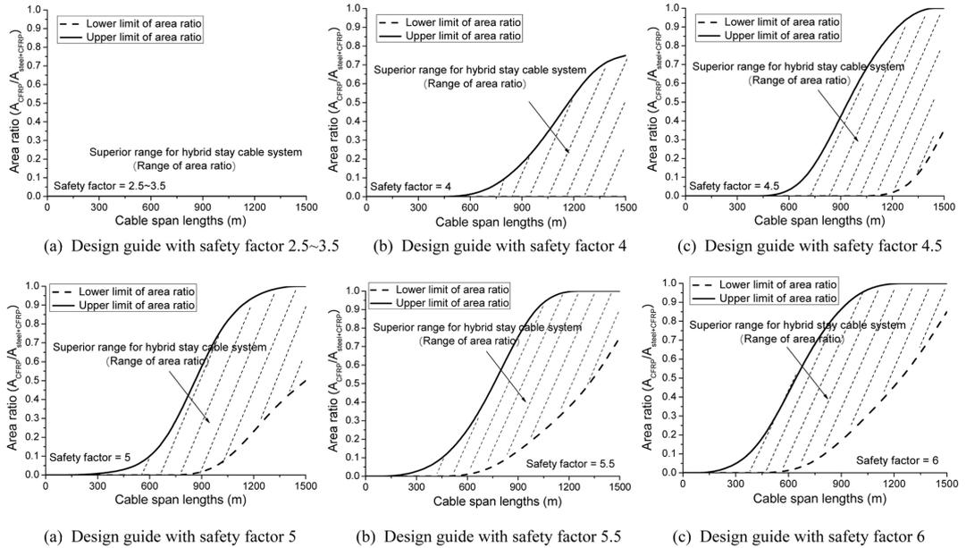
Fig. 12 Design guide for hybrid stay cable system based on design criterion 2 (price ratio = 10:1)
