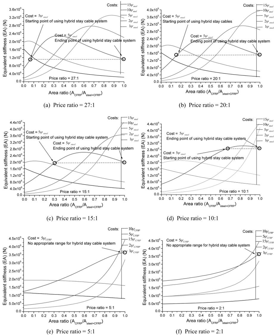
Fig. 13 Equivalent stiffness of stay cables with 700 m span length and different price ratios
