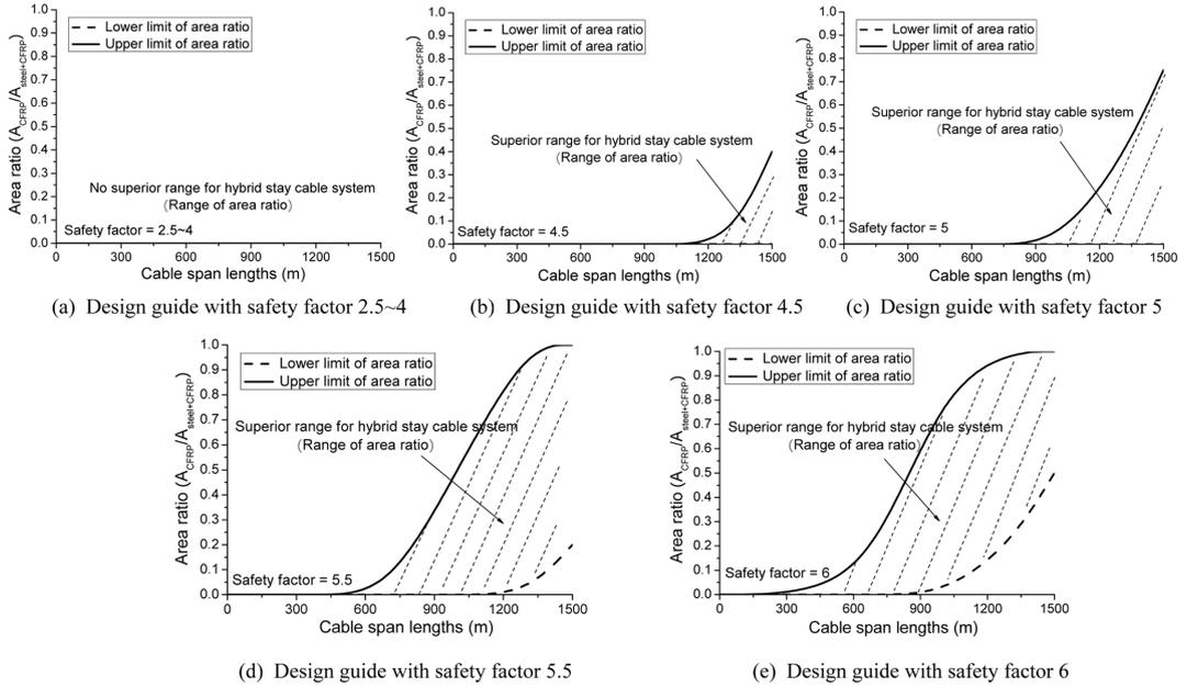
Fig. 11 Design guide for hybrid stay cable system based on design criterion 2 (price ratio = 15:1)
