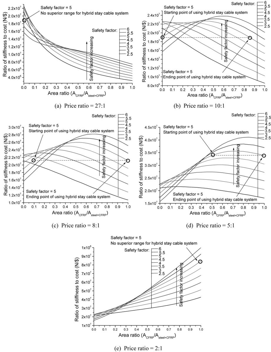
Fig. 10 Ratio of stiffness to cost for stay cables with 1000 m span length and different price ratios
