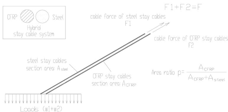
Fig. 6 Proposed hybrid stay cable system
