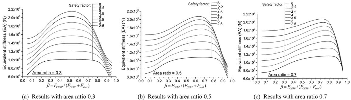
Fig. 18 Results for hybrid stay cable system with cable span length of 1000 m
