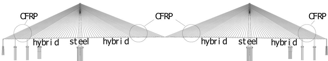
Fig. 19 Layout of the stay cables in the hybrid cable-stayed bridges
