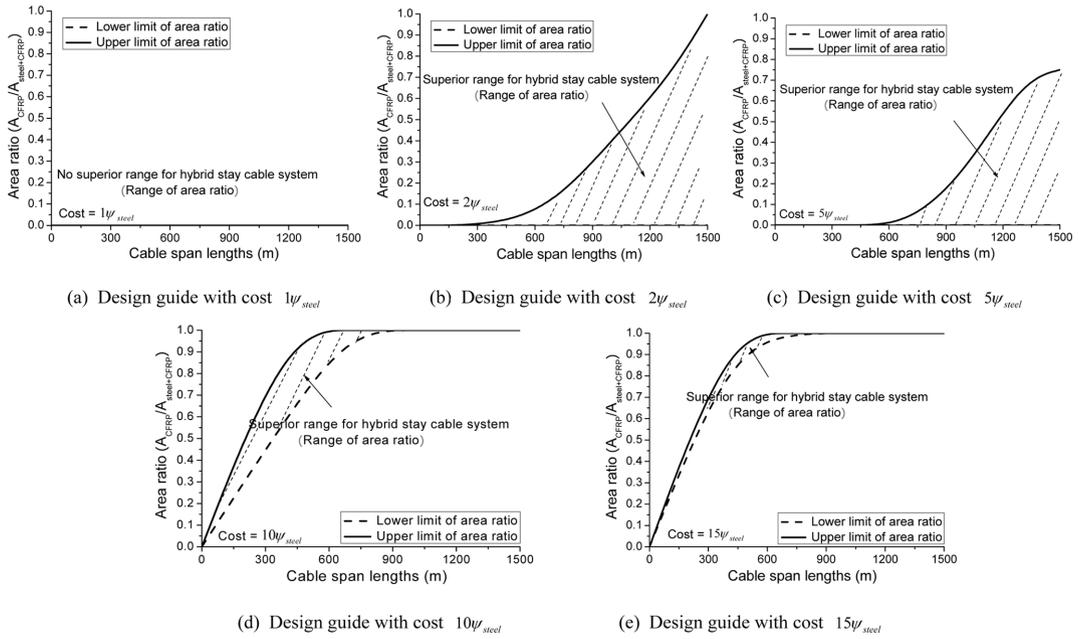
Fig. 15 Design guide for hybrid stay cable system based on design criterion 3 (price ratio = 15:1)
