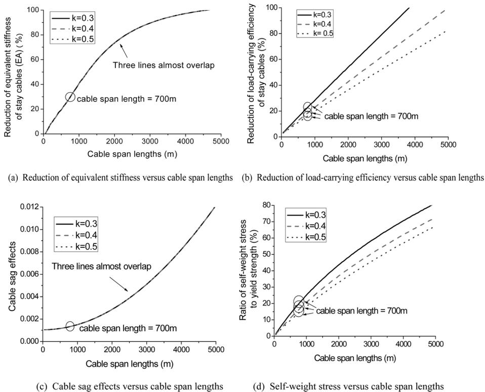
Fig. 3 Performance of pure steel stay cables versus cable span lengths
