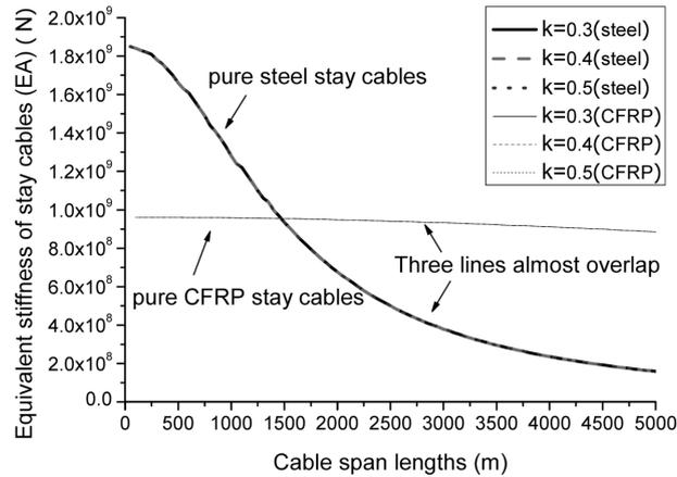
Fig. 5 Comparison for the equivalent stiffness (EA)
