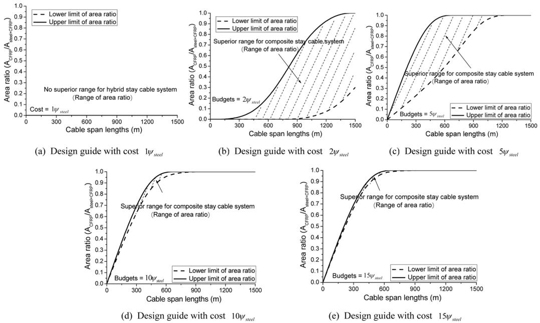
Fig. 16 Design guide for hybrid stay cable system based on design criterion 3 (price ratio = 10:1)
