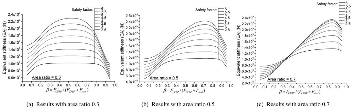
Fig. 17 Results for hybrid stay cable system with cable span length of 700 m
