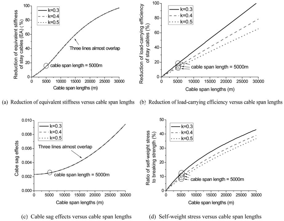
Fig. 4 Performance of pure CFRP stay cables versus cable span lengths
