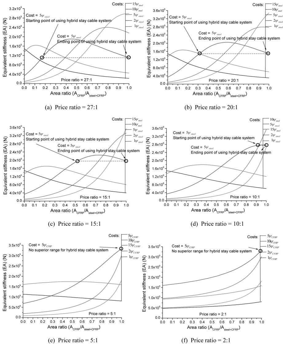
Fig. 14 Equivalent stiffness of stay cables with 1000 m span length and different price ratios
