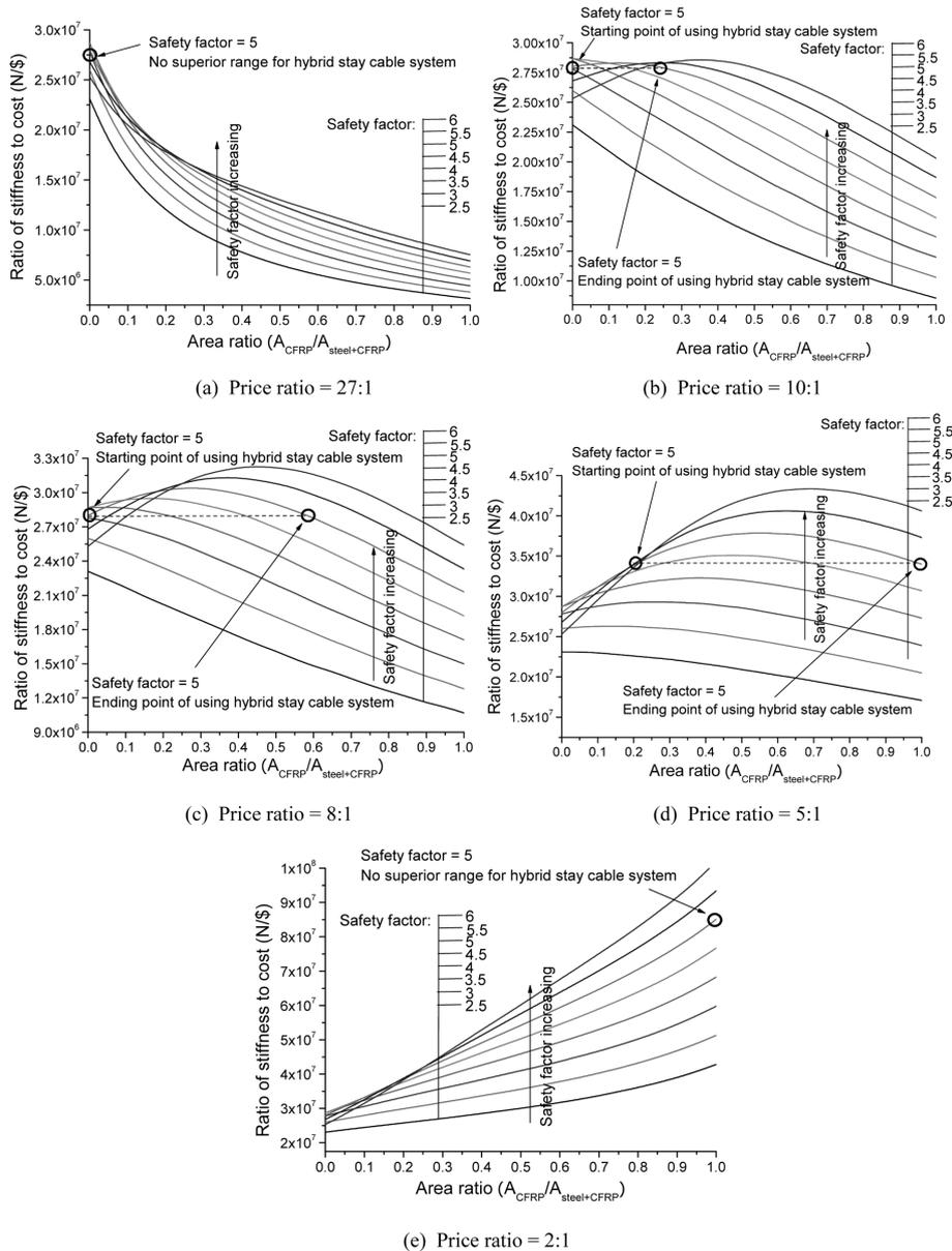
Fig. 9 Ratio of stiffness to cost for stay cables with 700 m span length and different price ratios
