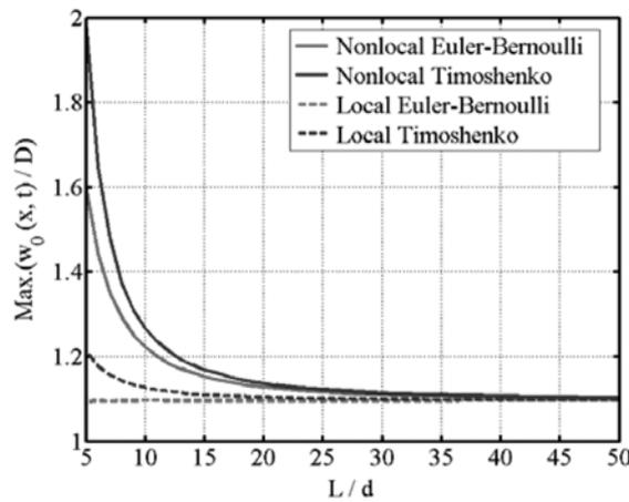
Fig. 3 The effects of aspect ratio of length to diameter  $L/d$  and beam models on the non-dimensional dynamic deflections for  $\alpha = 0.1$ ,  $k_w = 0$ ,  $e_0 a = 1 \text{ nm}$ .
