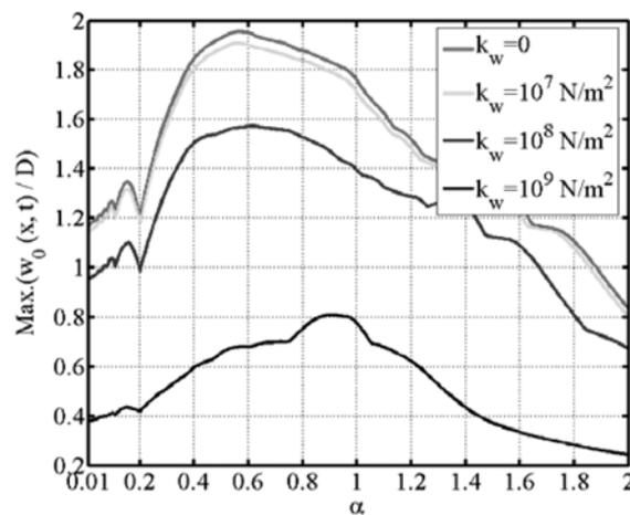
Fig. 6 The effect of the velocity parameter  $\alpha$  on the non-dimensional dynamic deflections for various values of  $k_w$  and  $L/d = 10, e_0a = 1$  nm.
