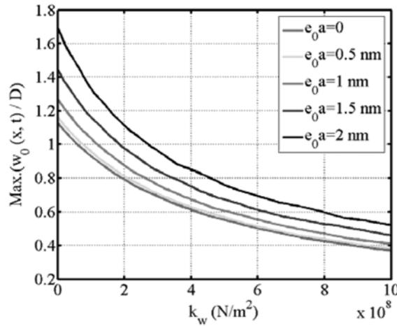
Fig. 7 The effect of the elastic medium constant  $k_w$  on the non-dimensional dynamic deflections for various values of  $e_0 a$  and  $\alpha = 0.1$ ,  $L / d = 1.0$ .
