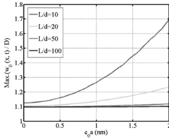
Fig. 4 The effect of the nonlocal parameter  $e_0a$  on the non-dimensional dynamic deflections for various values of  $L/d$  and  $\alpha = 0.1$ ,  $k_w = 0$ .
