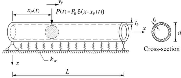
Fig. 1 A simply supported embedded SWCNT traversed by a moving load.
