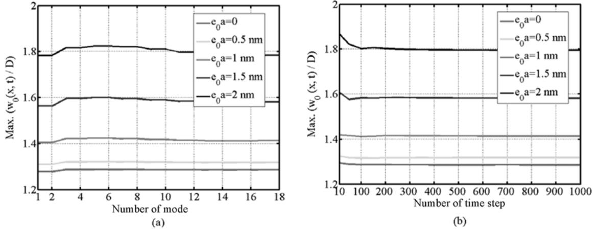
Fig. 2 The effects of the number of mode and of the time step on the non-dimensional dynamic deflections for various values of  $e_0 a$  and  $L/d = 10$ ,  $\alpha = 0.25$ ,  $k_w = 0$ .
