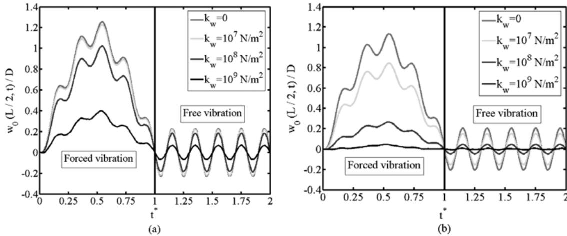
Fig. 8 Time history of the midspan displacements for various values of the elastic medium constant  $k_w$ ,  $\alpha = 0.1$ ,  $e_0\alpha = 1$  nm and a)  $L/d = 10$ , b)  $L/d = 20$ .
