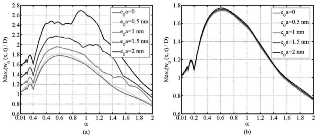
Fig. 5 The effect of the velocity parameter  $\alpha$  on the non-dimensional dynamic deflections for various values of  $e_0a$  and  $k_w = 0$ , a)  $L/d = 10$ , b)  $L/d = 50$ .
