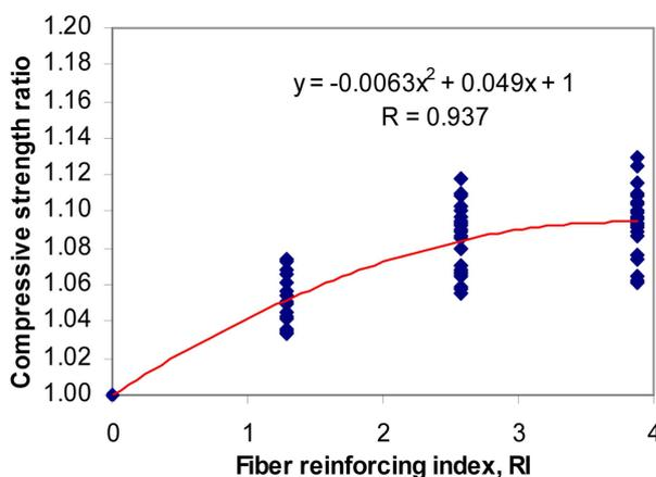
Fig. 1 Relationship between compressive strength ratio ( $f_{cf}/f_c$ ) and fiber reinforcing index (RI)
