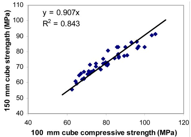
Fig. 4 Relationship between Compressive strengths of 150 mm cube and 100 mm cube of fiber reinforced concretes
