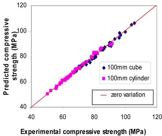
Fig. 3 Correlation of 100 mm cube and 100 mm dia. cylinder strengths (MPa) with the predicted values of compressive strengths (MPa)
