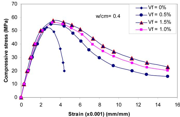
Fig. 5 Typical stress-strain curve for SF concrete and steel fiber reinforced concrete ( $w/cm = 0.40$ , SF content = 10%)
