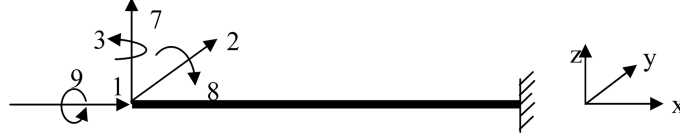
Fig. 2 A cantilever model for calculating the relations between the nodal actions and basic deformation parameters
