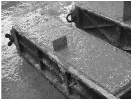
Fig. 1 Fresh concrete in the mold (100 mm × 100 mm × 400 mm)
