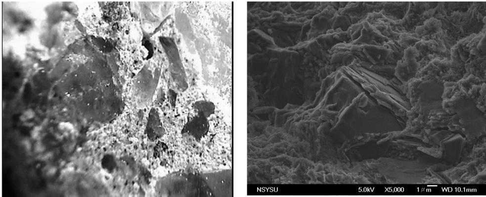
Fig. 10 The OM and SEM picture for WGCLSM
