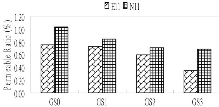
Fig. 8 Permeable ratio of different glass sand replacement amount of general type and the early-high-strength type WGCLSM
