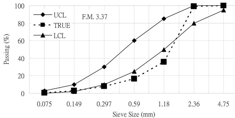
Fig. 2 Glass sand composition curve
