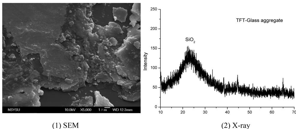
Fig. 3 The SEM picture and X-ray diffraction graphs for LCD glass sand
