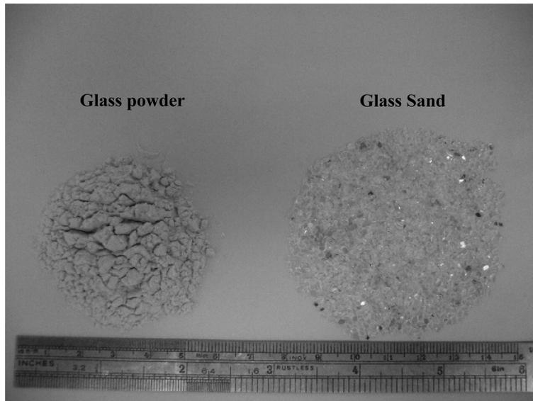
Fig. 1 Glass powder and glass sand of LCD
