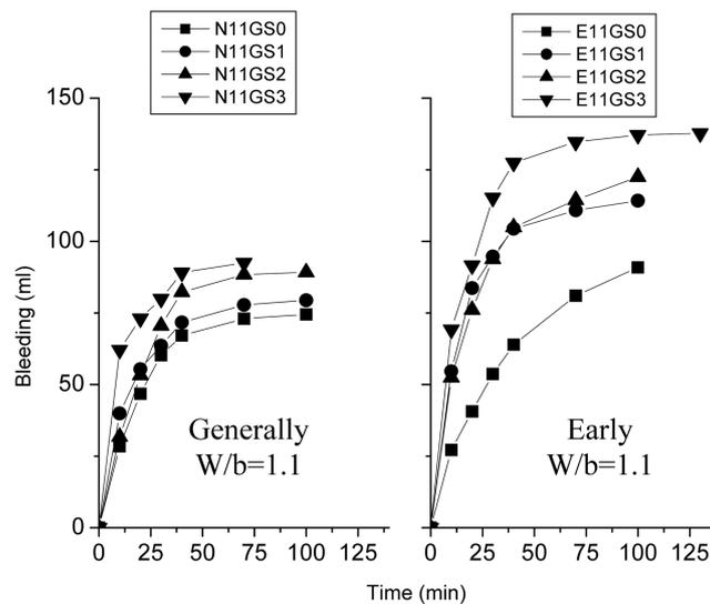
Fig. 4 Accumulated bleeding amount of different glass sand replacement amount of general type and the early-high-strength type WGCLSM
