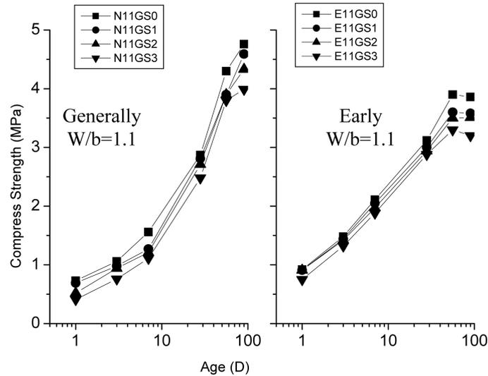
Fig. 5 Compressive strength of different glass sand replacement amount of general type and the early-high-strength type WGCLSM
