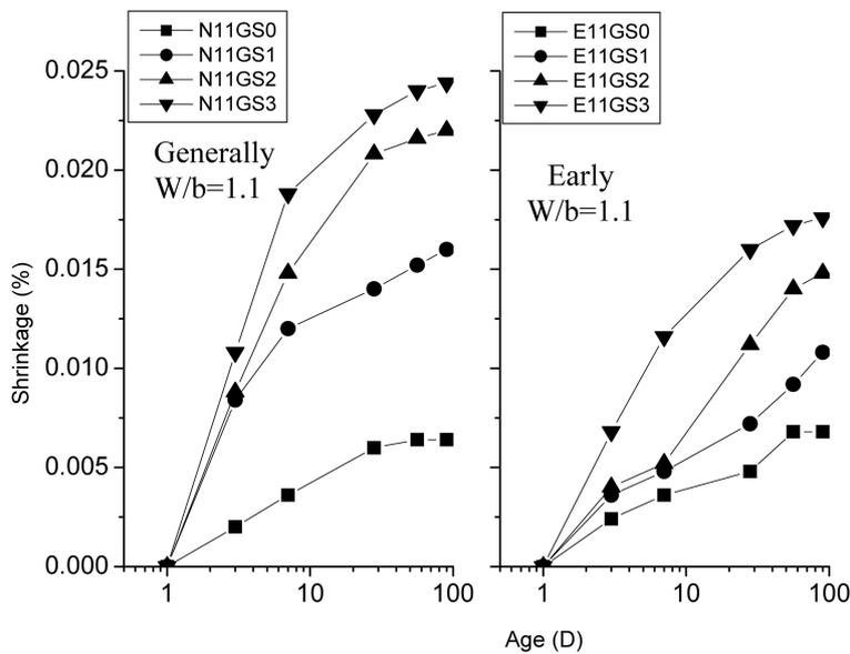
Fig. 9 Length variation of different glass sand replacement amount of general type and the early-high-strength type WGCLSM
