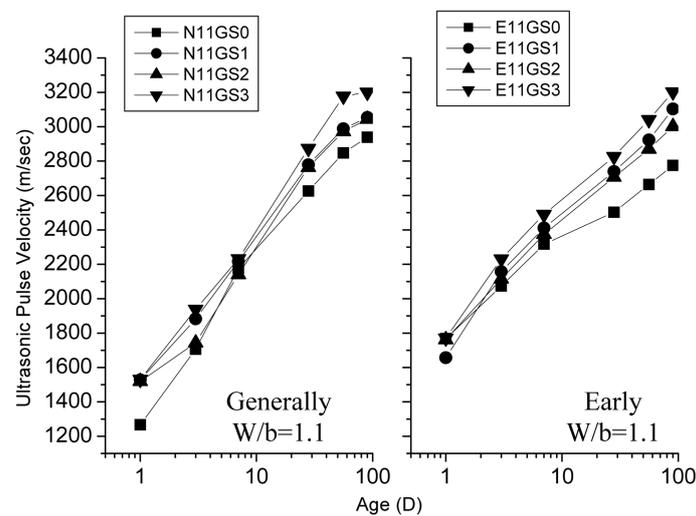
Fig. 7 Ultrasonic curve of different glass sand replacement amount of general type and the early-high-strength type WGCLSM
