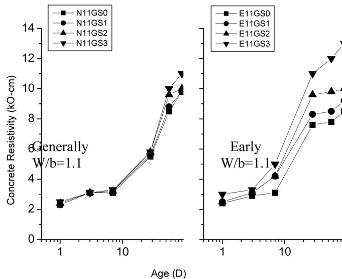
Fig. 6 Electrical resistivity of different glass sand replacement amount of general type and the early-high-strength type WGCLSM
