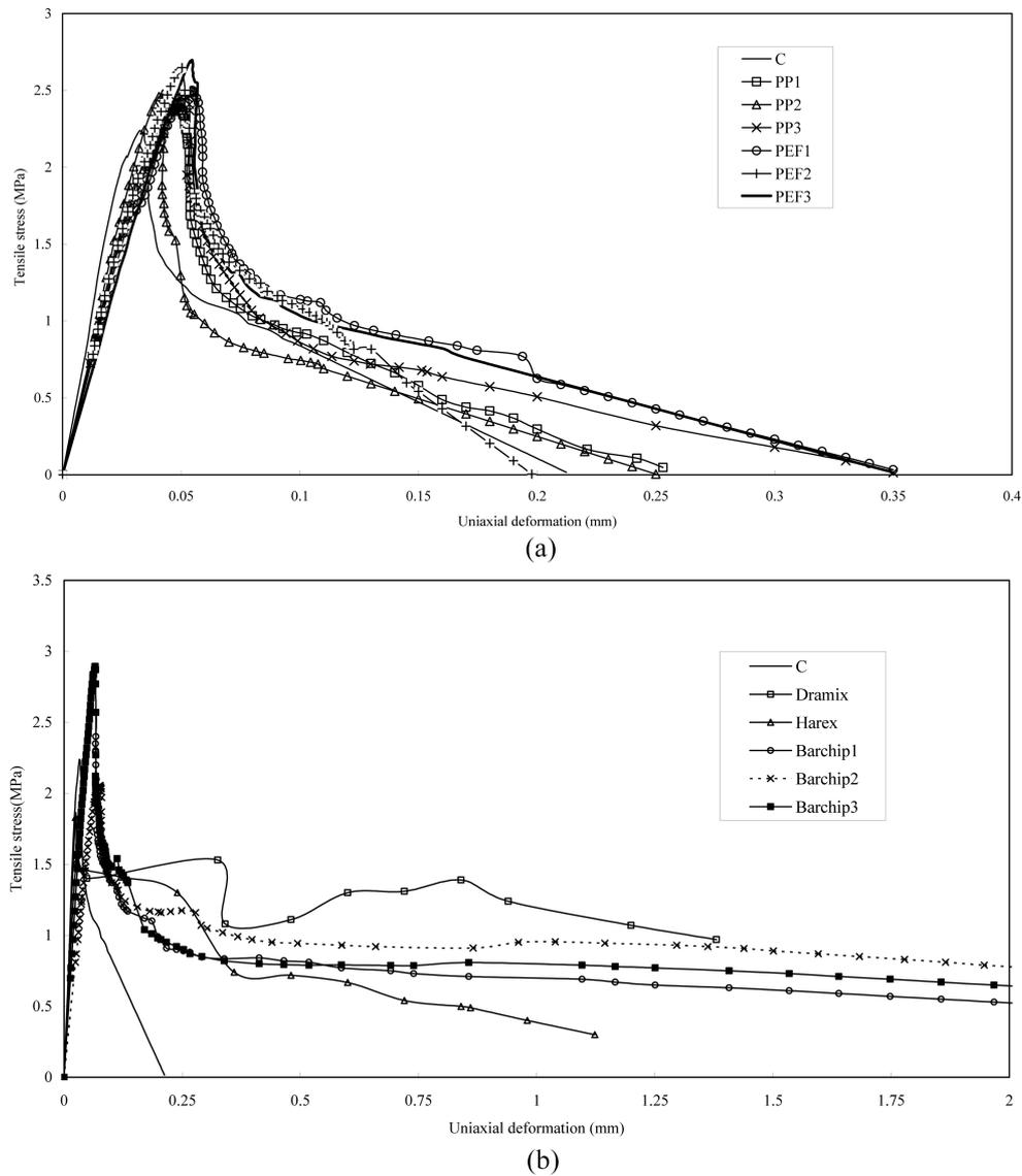
Fig. 2 Axial stress-deformation curves of macro-fiber reinforced concrete in uniaxial tension
