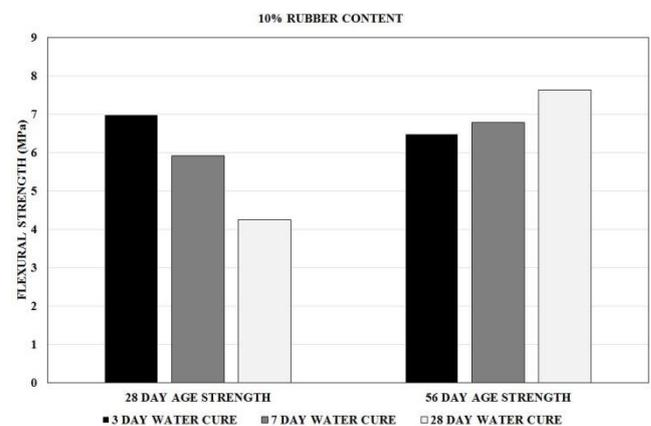
Fig. 11 10% SBR replacement effect on flexural strength change with the curing time
