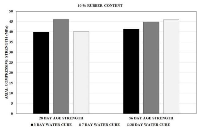
Fig. 7 10% SBR replacement effect on compressive strength change with the curing time
