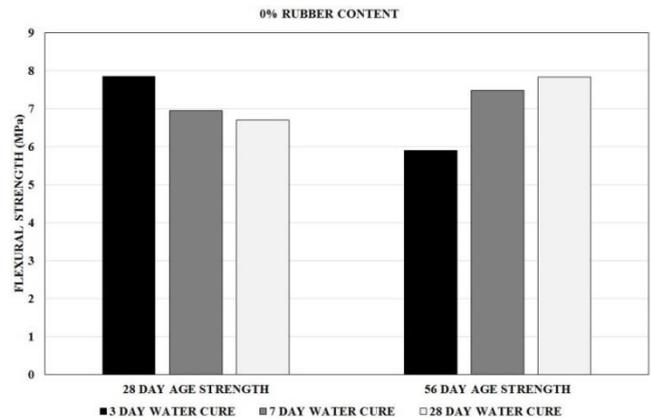
Fig. 10 Control mix flexural strength change with the curing time
