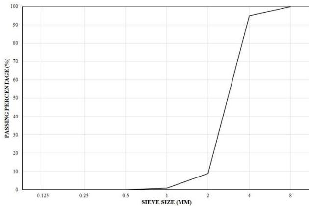
Fig. 2 SBR particles sieve analysis
