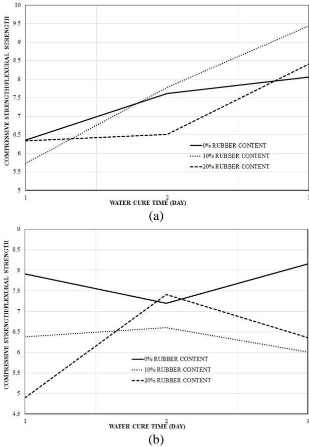
Fig. 16 Compressive strength/ flexural strength ratio (a) 28-days age test (b) 56-days age test
