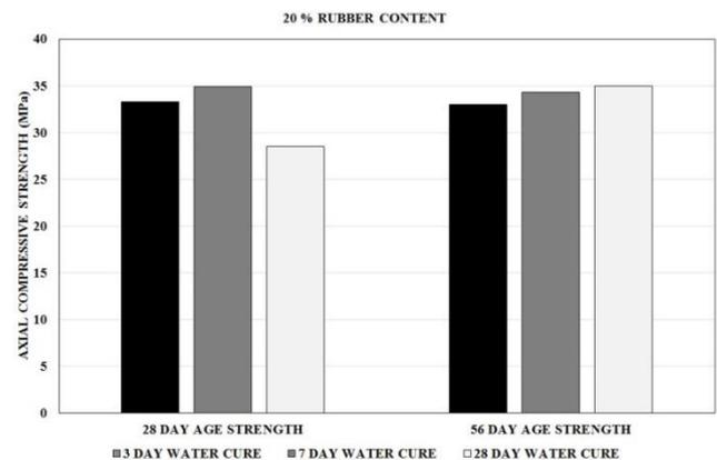
Fig. 8 20% SBR replacement effect on compressive strength change with the curing time
