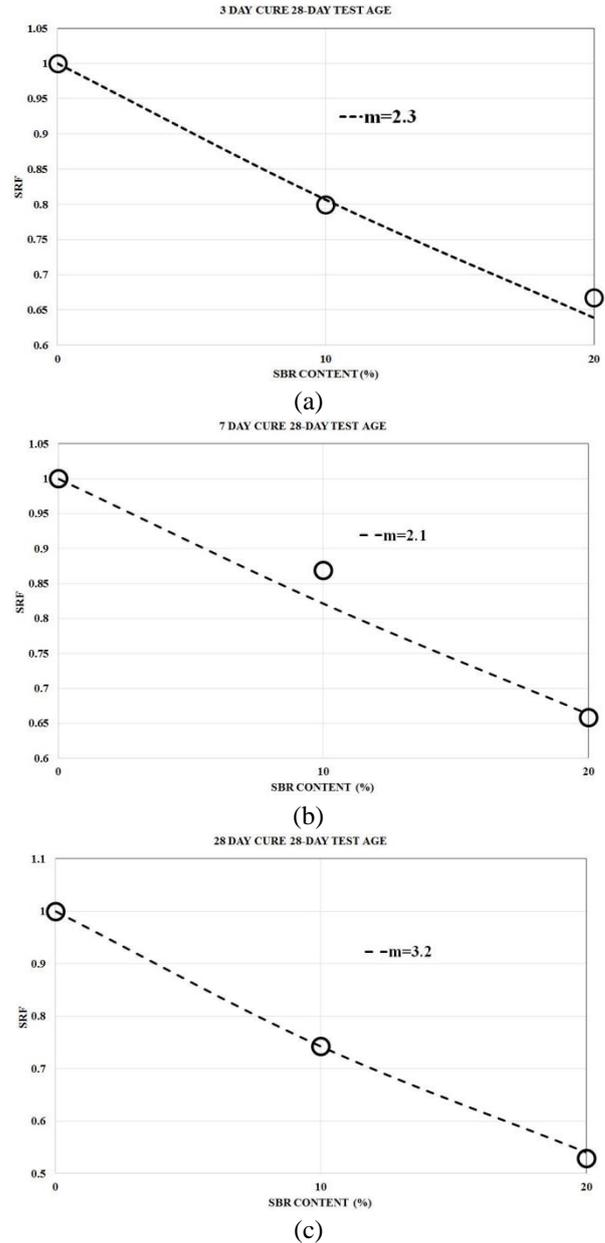
Fig. 17 Curves for proposed SRF characteristic function at 28-days test age (a) 3-days water cure (b) 7-days water cure (c) 28-days water cure
