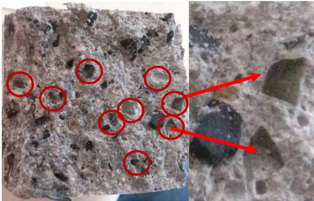
Fig. 9 Bond loss between the SBR particles and cement paste
