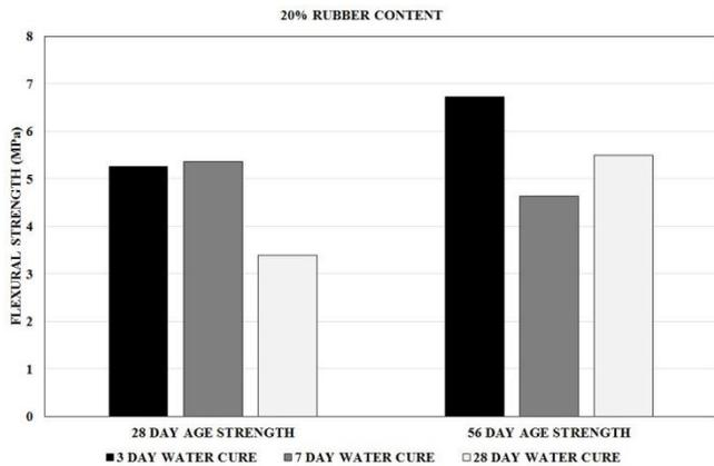
Fig. 12 20% SBR replacement effect on flexural strength change with the curing time
