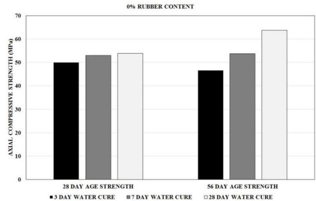
Fig. 6 Control mix compressive strength change with the curing time
