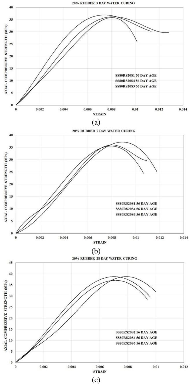
Fig. 15 20% SBR replacement effect on compressive strength-strain graph (a) 3-days water curing (b) 7-days water curing (c) 28-days water curing at the age of 56 days
