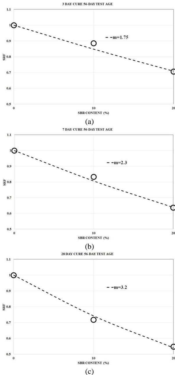
Fig. 18 Curves for proposed SRF characteristic function at 56-days test age (a) 3-days water cure (b) 7-days water cure (c) 28-days water cure
