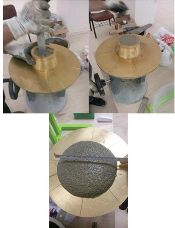
Fig. 3 Slump flow test according to ASTM C1437 (ASTM 2001)
