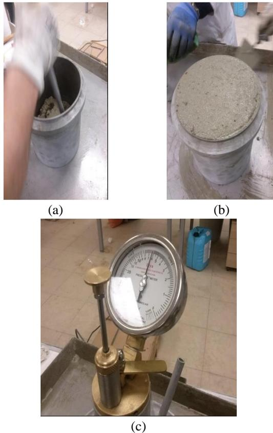
Fig. 5 (a) Mortar were placed, (b) Density measurement, (c) Air content measurement
