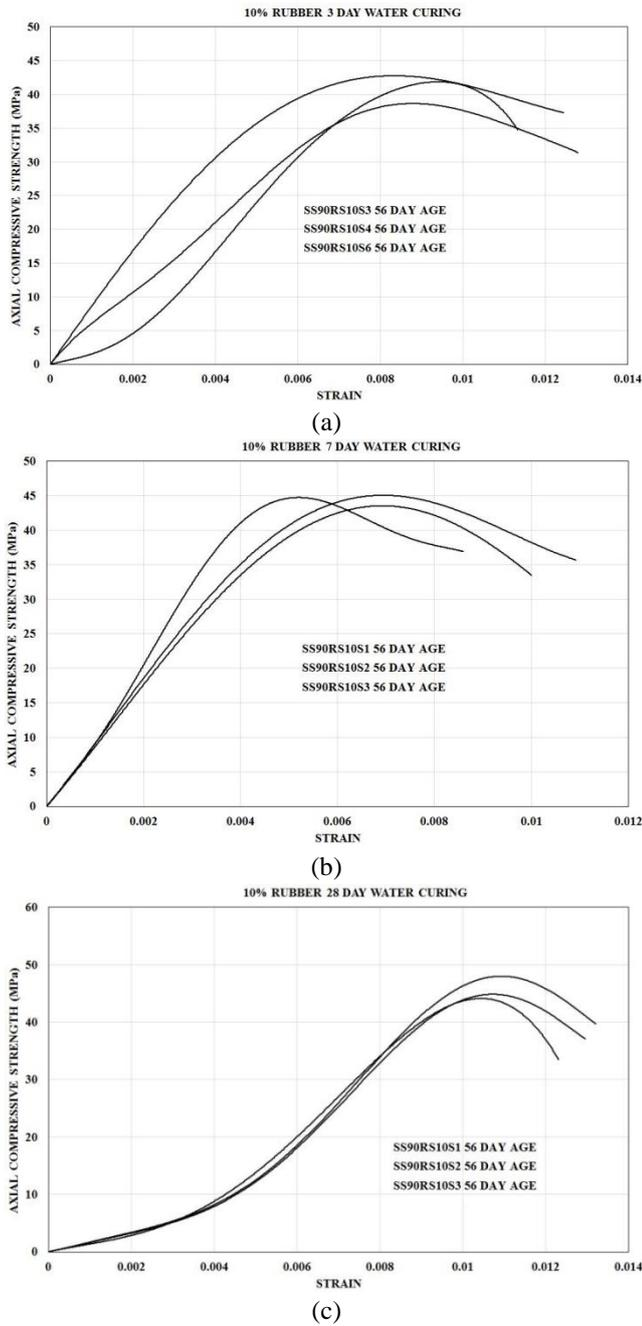
Fig. 14 10% SBR replacement effect on compressive strength-strain graph (a) 3-days water curing (b) 7-days water curing (c) 28-days water curing at the age of 56 days
