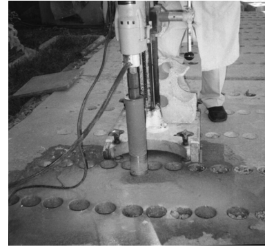
Fig. 2 Extraction of core samples for testing
