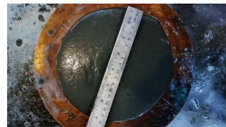
(c) Accessory apparatus for mortar flow testing
