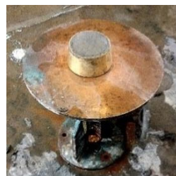
(b) Mortar flow test
