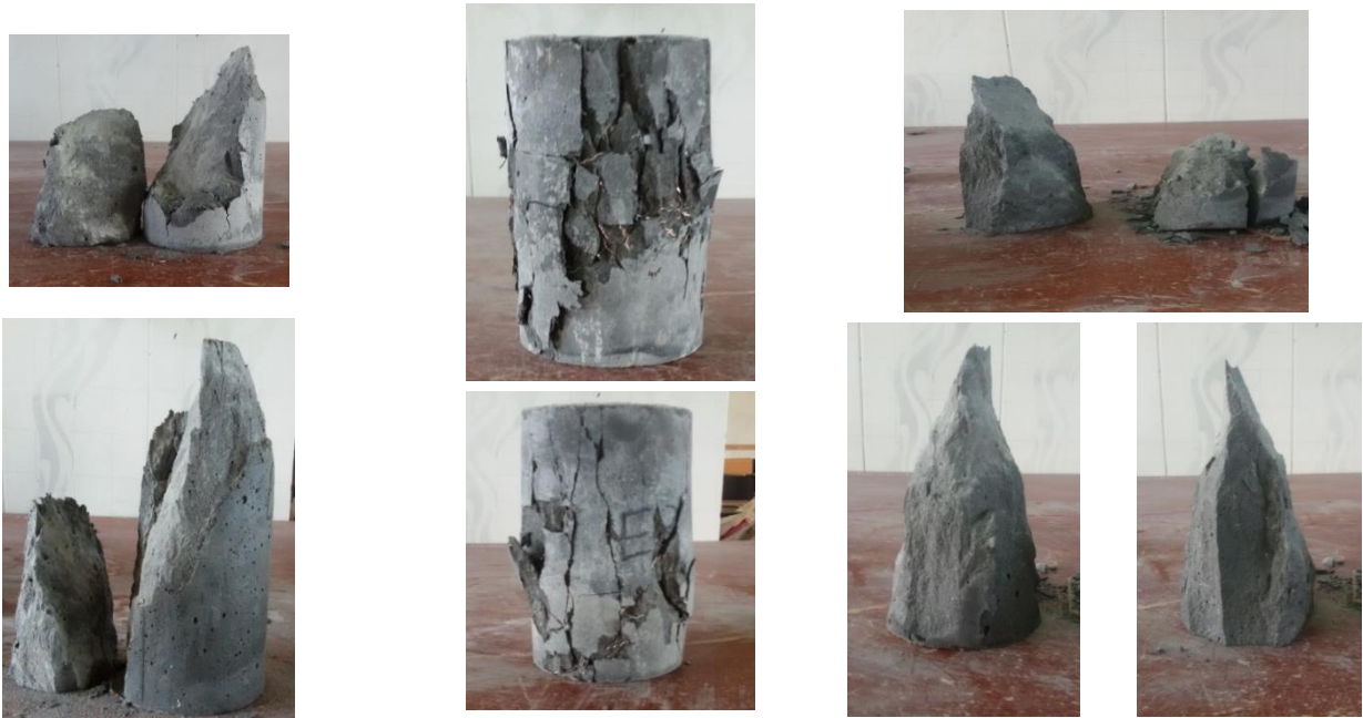
(a) Concrete containing PVA fibers
