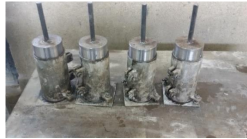
(a) Placement of steel lids on concrete specimens
