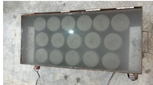
(b) Curing box and specimens under heat treatment
