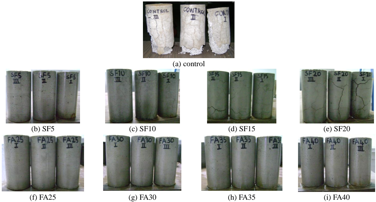
Fig. 5 Images of the SCM mixtures after 90 freeze-thaw cycles
