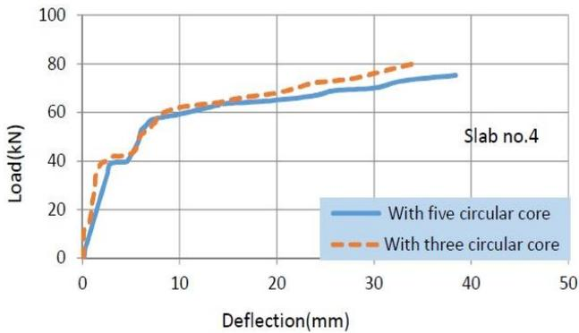
Fig. 25 Effect of number of cores on the behavior of lightweight aggregate hollow circular core slab
