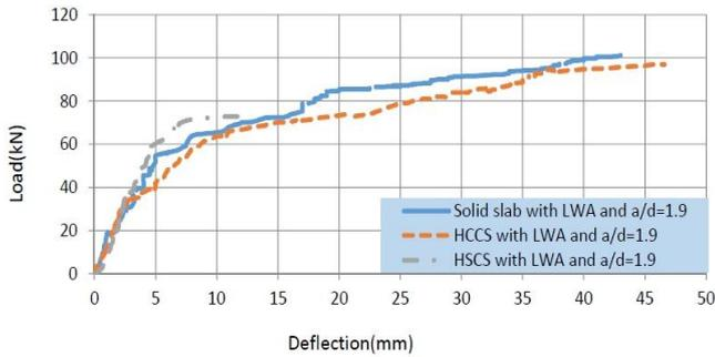
Fig. 14 Load-deflection relationship of solid and hollow core slabs
