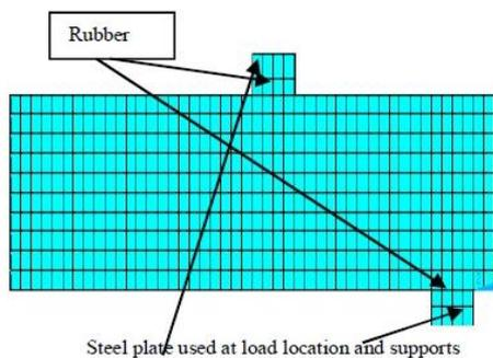
Fig. 3 Rubbers and steel plates for quarter of slab model that used in analysis
