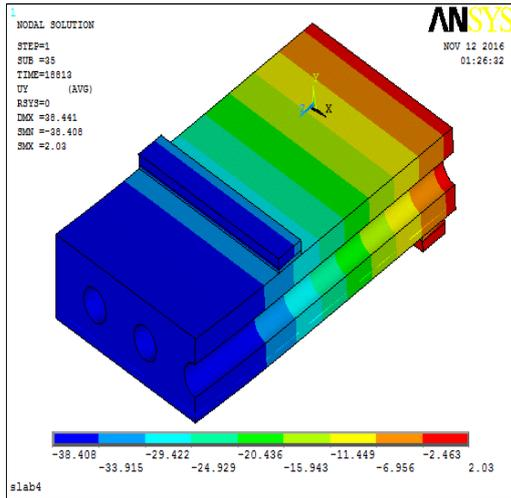
Fig. 20 Deflection contours in y-direction of tested slab no.4 at ultimate load
