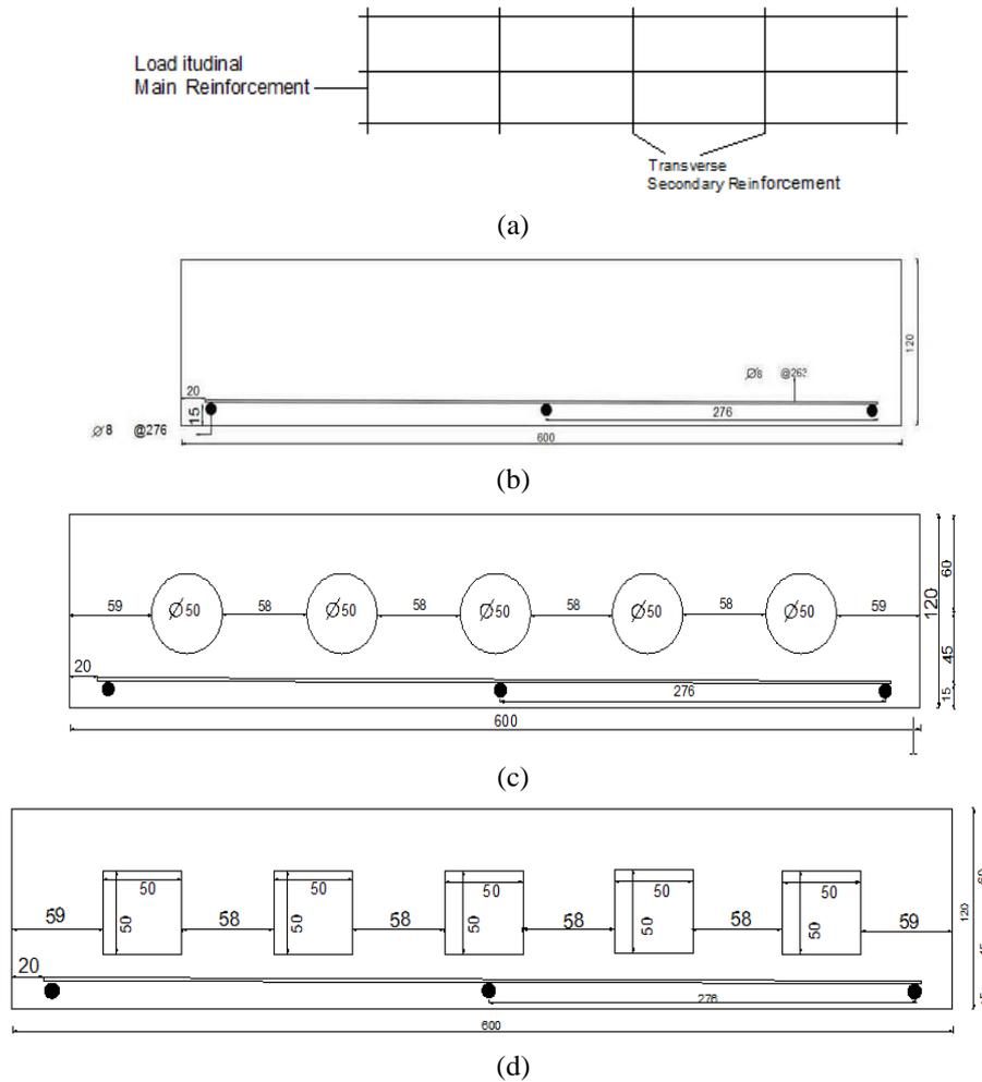
Fig. 1 (a) Specimens geometry and details, (b) Solid slab (c) and (d) Hollow core slabs ( All dimensions are in mm)
