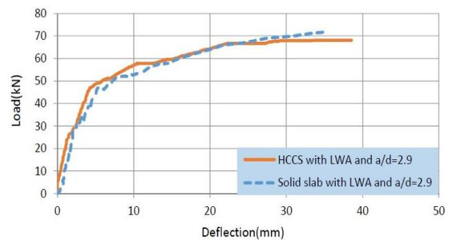
Fig. 13 Load-deflection relationship of solid and hollow circular core slabs
