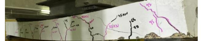
Fig. 9 Crack pattern at ultimate load for slab no. 6
