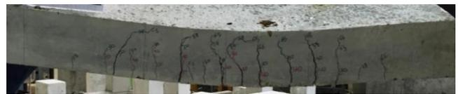
Fig. 7 Crack pattern at ultimate load for slab no. 4
