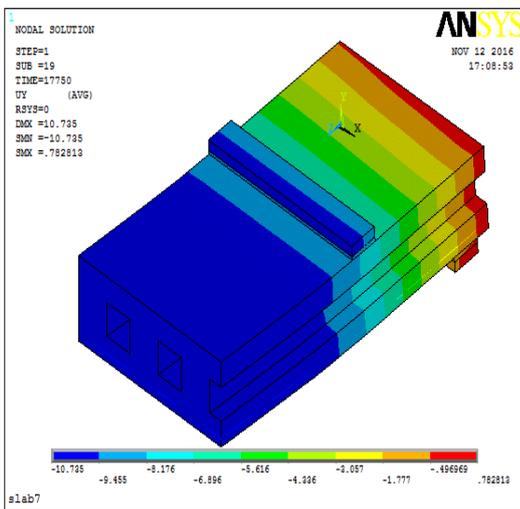
Fig. 21 Deflection contours in y-direction of tested slab no.7 at ultimate load
