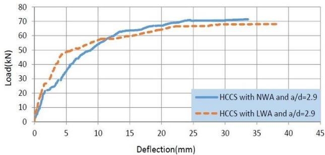
Fig. 15 Load-deflection relationship of normal and lightweight concrete hollow core slabs
