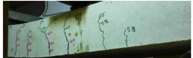
Fig. 22 Crack pattern at ultimate load for slab no.4
