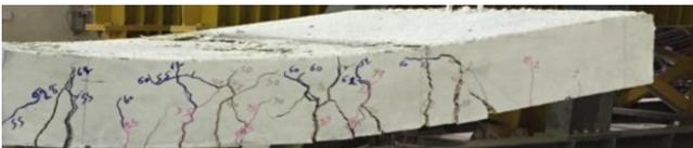
Fig. 5 Crack pattern at ultimate load for slab no. 2
