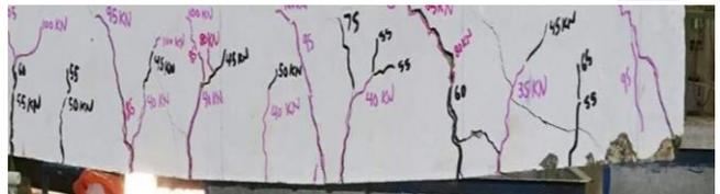
Fig. 23 Crack pattern at ultimate load for slab no. 5
