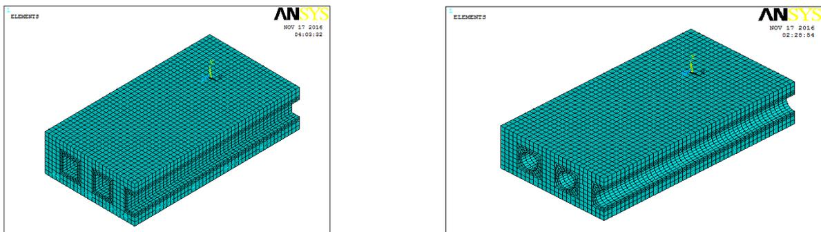
Fig. 2 Mesh of quarter of circular and square hollow core slab
