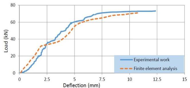
Fig. 19 Experimental and finite element load - deflection curves for slab no.7
