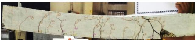
Fig. 6 Crack pattern at ultimate load for slab no. 3
