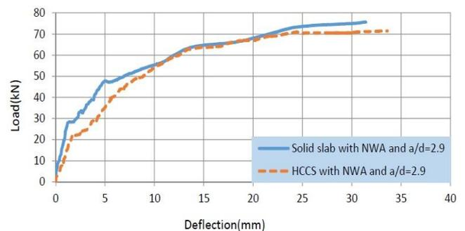
Fig. 12 Load-deflection relationship of solid and hollow circular core slabs
