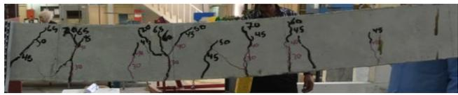
Fig. 8 Crack pattern at ultimate load for slab no. 5
