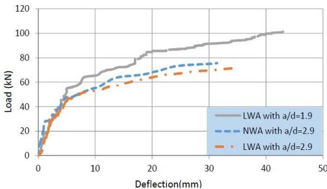
Fig. 11 Load-deflection relationship of solid slabs for different  $a/d$  ratios
