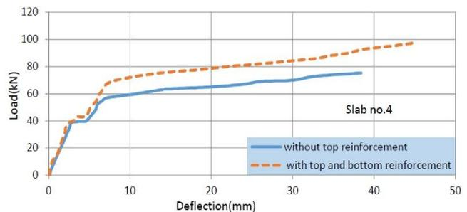
Fig. 24 Effect of top reinforcement layer on the behavior of lightweight aggregate hollow circular core slab
