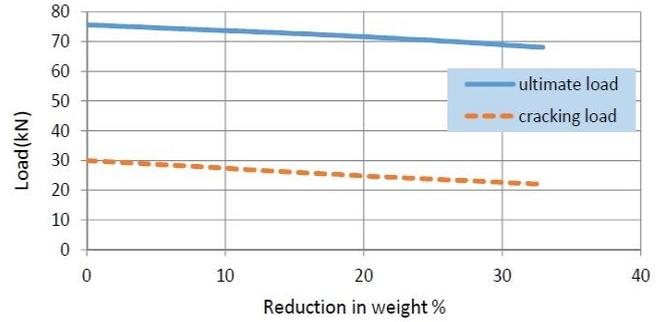
Fig. 17 Relationship between reduction in weight and applied loads (cracking and ultimate loads)
