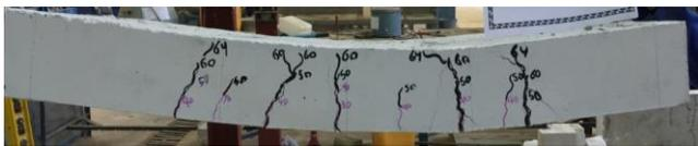
Fig. 4 Crack pattern at ultimate load for slab no. 1
