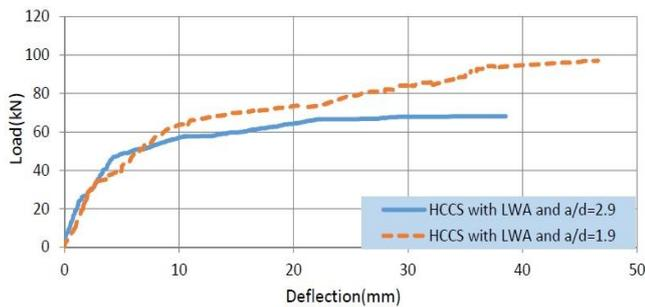
Fig. 16 Load-deflection relationship of hollow core slabs with different in  $a/d$  ratios
