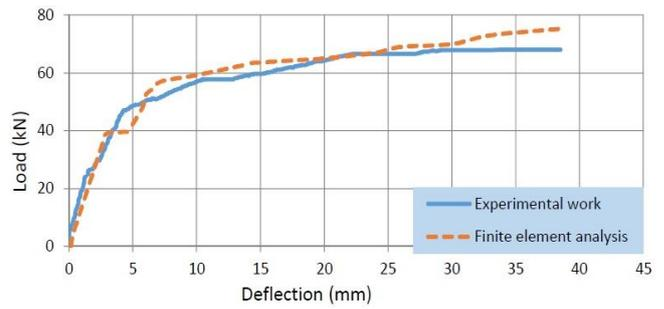
Fig. 18 Experimental and finite element load - deflection curves for slab no.4
