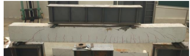
Fig. 18 Crack pattern obtained by experiment
