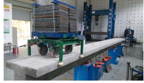
Fig. 2 Loaded vehicle moving on continuous RC beam
