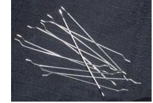
Carbon steel fiber is produced from high-strength cold-drawn steel wire; conform to ASTM 820, widely used for concrete reinforcement
