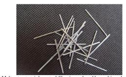
Melt extract stainless steel fiber is produced by melting elements in a crucible. A flywheel is then introduced to the crucible and droplets of molten metal are spun into the open air and hardened
