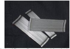
Glued steel fibers are filaments of wire, deformed and cut to lengths, for reinforcement of concrete, with hooked ends. It is easy to separate in the mixer and can avoid balling in concrete matrix
