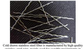
stainless steel wire, mainly used for castable requirements in refractory field
