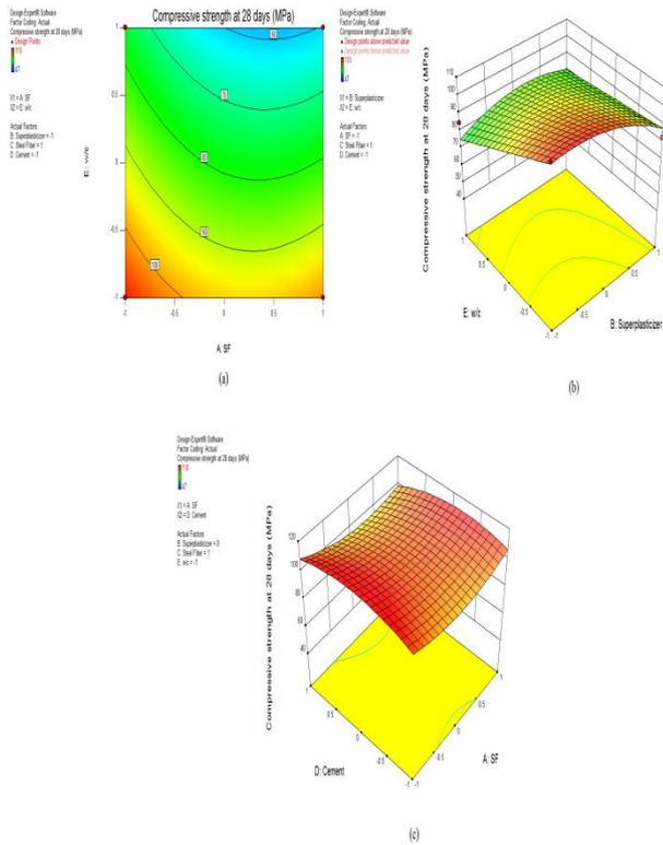
Fig. 5 Contour plot and response surface of 28 days compressive strength
