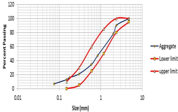
Fig. 1 Sieve analysis of lime stone
