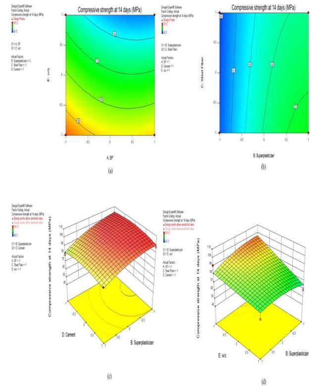
Fig. 4 Contour plot and response surface of 14 days compressive strength
