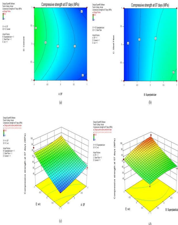
Fig. 3 Contour plot and response surface of 7 days compressive strength
