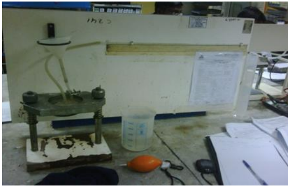
Fig. 4 Initial surface absorption test
