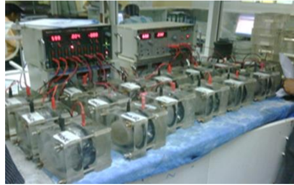
Fig. 1 Resist chloride ion penetration test
