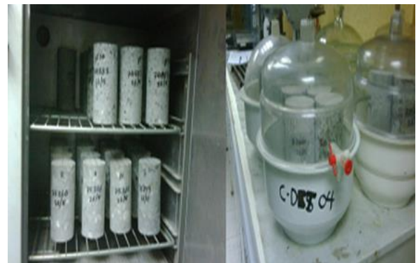
Fig. 3 Water absorption test
