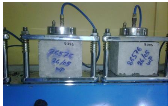
Fig. 2 Water permeability test
