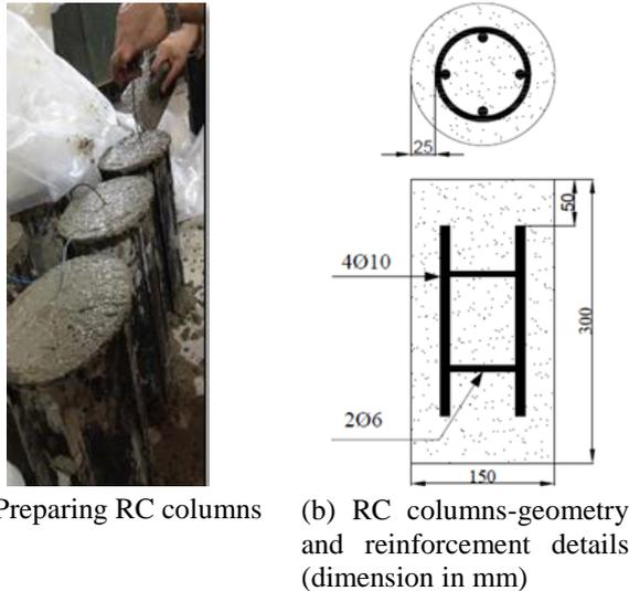
Fig. 1 Reinforced concrete specimens
