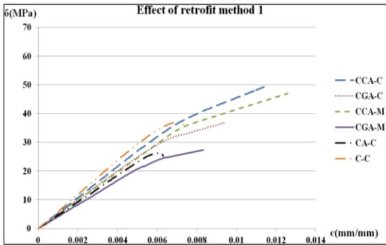
(a) Axial stress-strain curves of strengthened specimens
