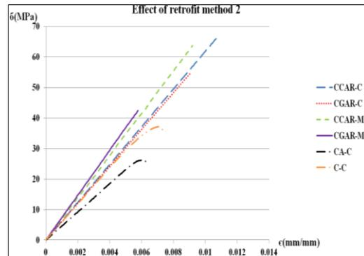
(a) Axial stress-strain curves of strengthened specimens
