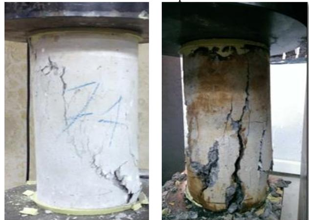
(b) Failure mode of non-corroded RC columns (c) Failure mode of corroded RC columns
