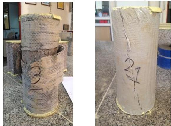
(b) Failure mode of CCAR-M(c) Failure mode of CGAR-M
