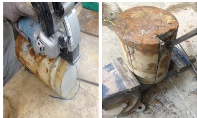
(a) Cutting corroded concrete (b) Removing corroded concrete
