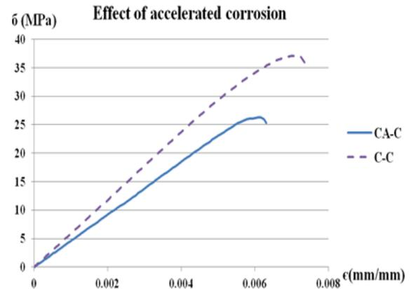
(a) Axial stress-strain curves of non-corroded and corroded RC columns before exposure
