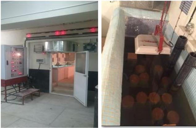
(a) Exterior view of the marine simulator (b) Specimens placed in tidal pool
