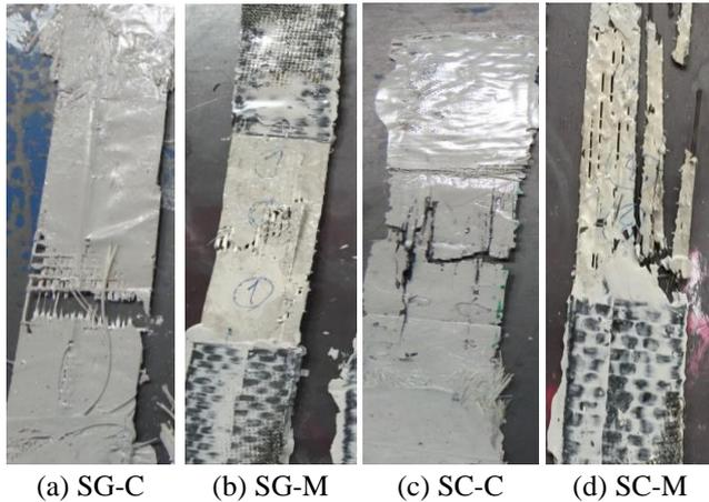
Fig. 6 Failure mode of FRP sheets
