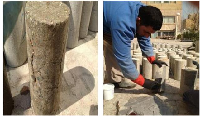
(a) Cleaned specimens (b) Applying primer
