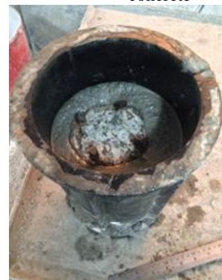
(c) Replacing corroded concrete by self-compacted mortar
