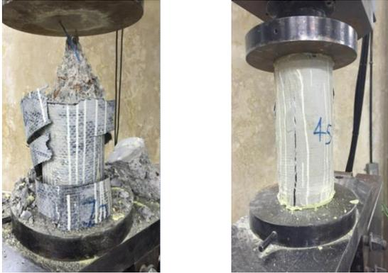
(b) Failure mode of CCA-M (c) Failure mode of CGA-M
