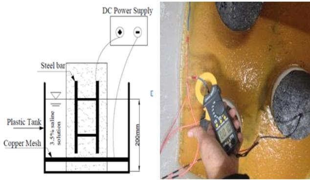
(a) Schematic presentation of the accelerated corrosion process (b) Accelerated corrosion process in the laboratory
