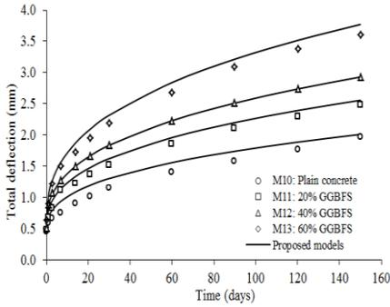
Fig. 7 Comparison between predicted and experimental total deflection for mix group M1
