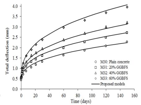
Fig. 9 Comparison between predicted and experimental total deflection for mix group M3
