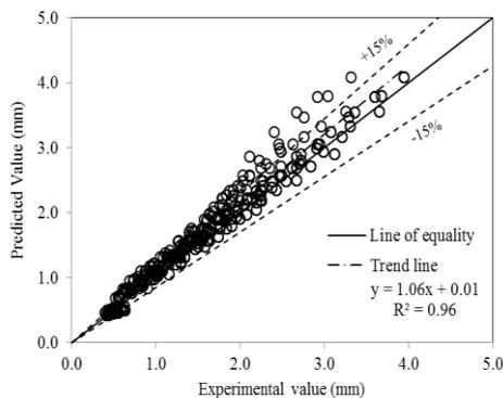
Fig. 12 Comparison between predicted and experimental total deflection for all data points including the data of previous study (Shariq *et al.* 2013)
