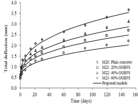
Fig. 8 Comparison between predicted and experimental total deflection for mix group M2
