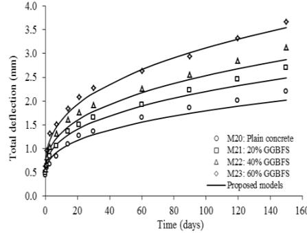
Fig. 8 Comparison between predicted and experimental total deflection for mix group M2
