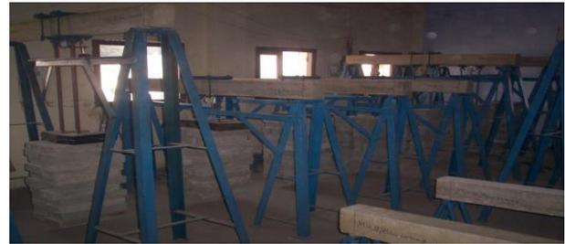
Fig. 3 RC beam specimens under test
