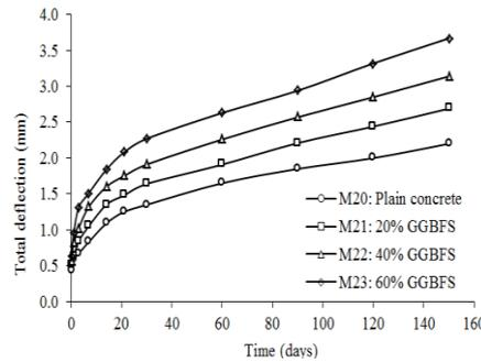
Fig. 5 Mid-span deflection of RC beams of mix group M2
