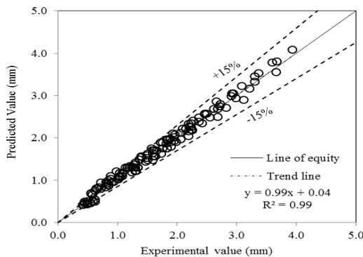
Fig. 11 Comparison between predicted and experimental total deflection for all data points of the present study
