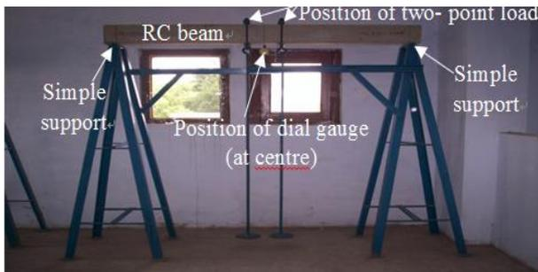
Fig. 2 Test setup for the measurement of time-dependent deflection of RC beam
