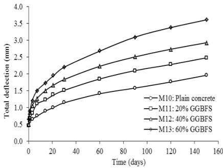
Fig. 4 Mid-span deflection of RC beams of mix group M1
