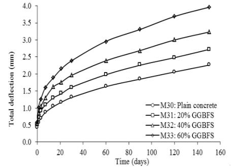
Fig. 6 Mid-span deflection of RC beams of mix group M3
