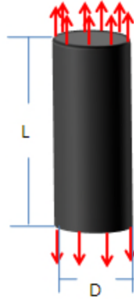
Fig. 1 Schematic picture of the loading of the specimen in a direct tension test
