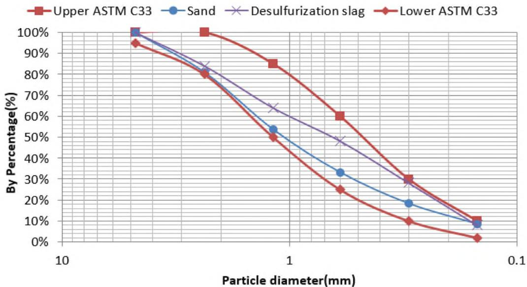
Fig. 1 Size distribution of natural fine aggregate and desulphurization slag
