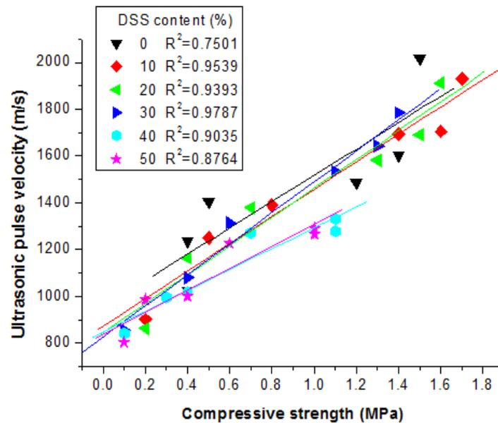
Fig. 7 Linear regression relationships between the compressive strength and ultrasonic pulse velocity of RMSM
