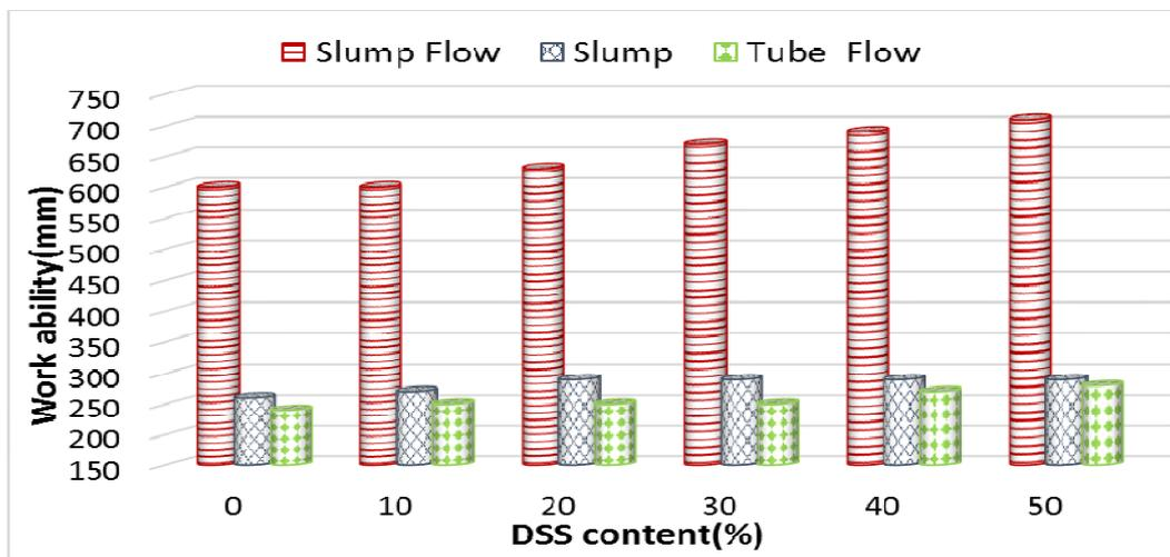
Fig. 2 Workability of RMSM with desulphurization slag replacement
