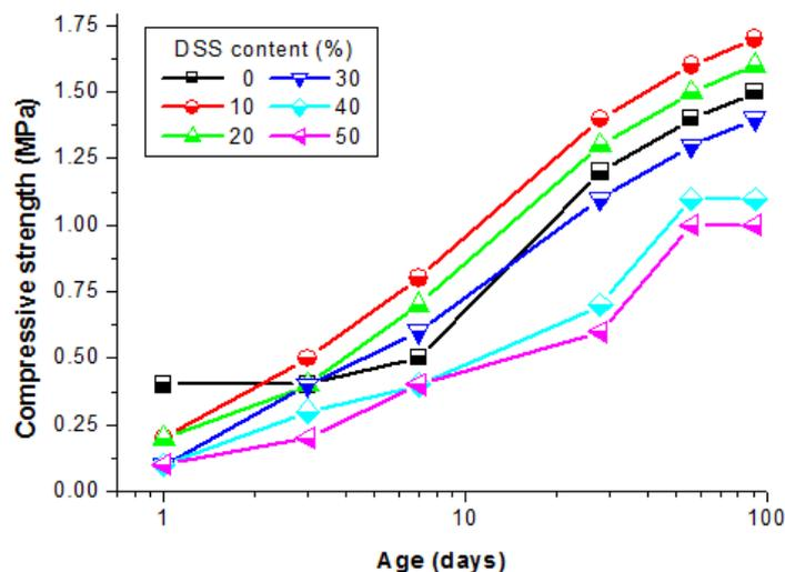
Fig. 2 Relationship between the age and compressive strength of RMSM
