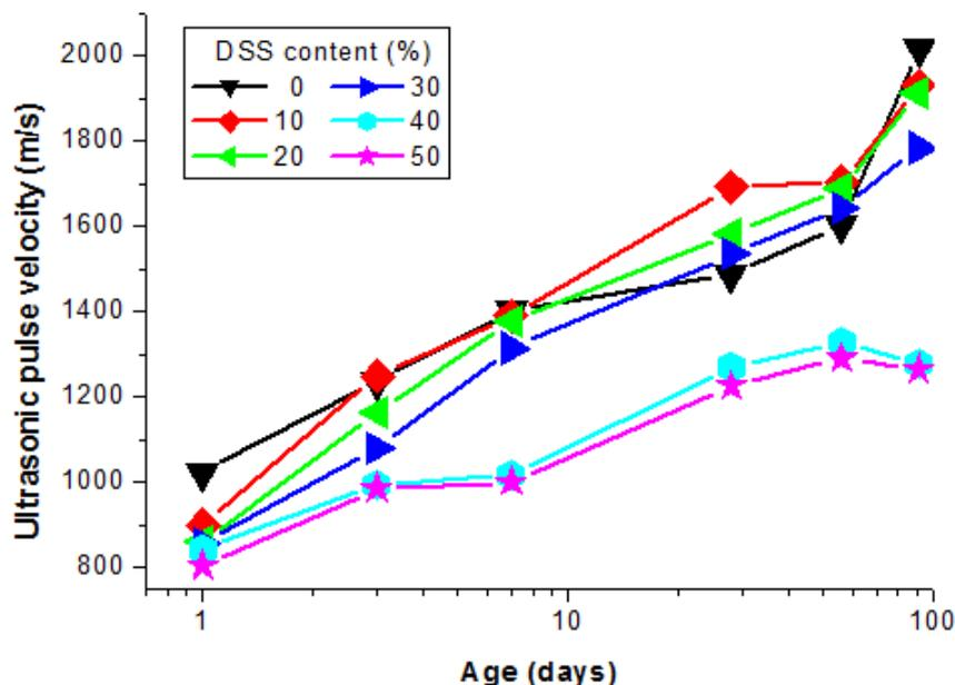
Fig. 6 Relationship between the age and ultrasonic pulse velocity of RMSM
