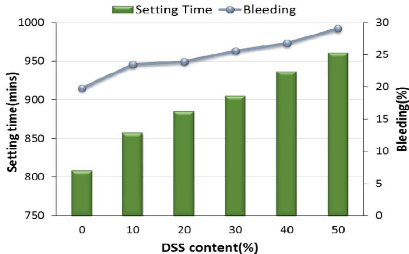
Fig. 1 Relationship between the RMSM setting time and bleeding
