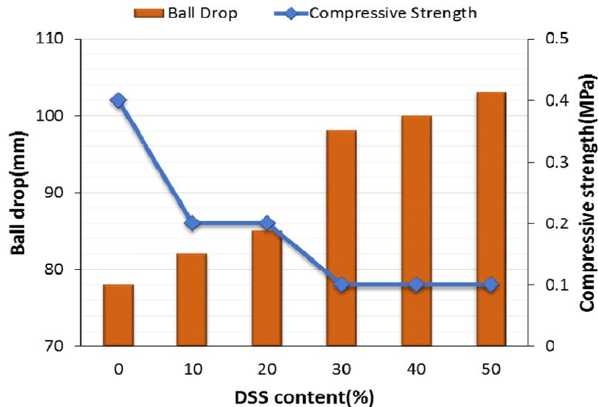
Fig. 3 Relationship between the ball drop and one-day compressive strength of various mixed proportion groups of RMSM
