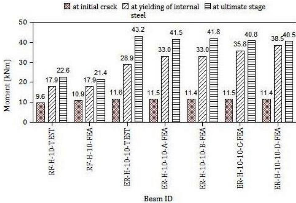
Fig. 8 Comparison of moment at critical stages– H-10 series
