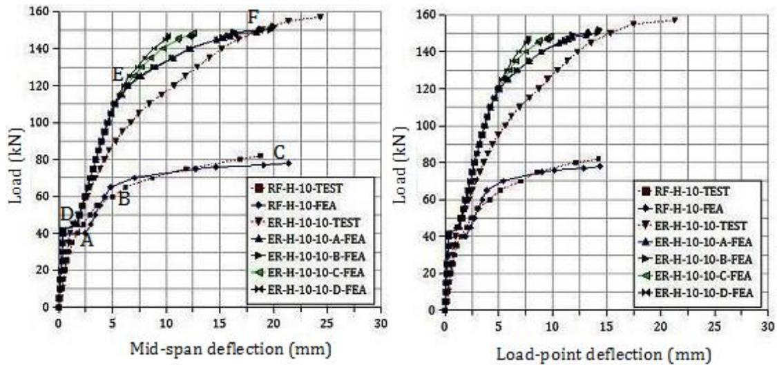
Fig. 4 Load versus deflection for beams in H-10 series
