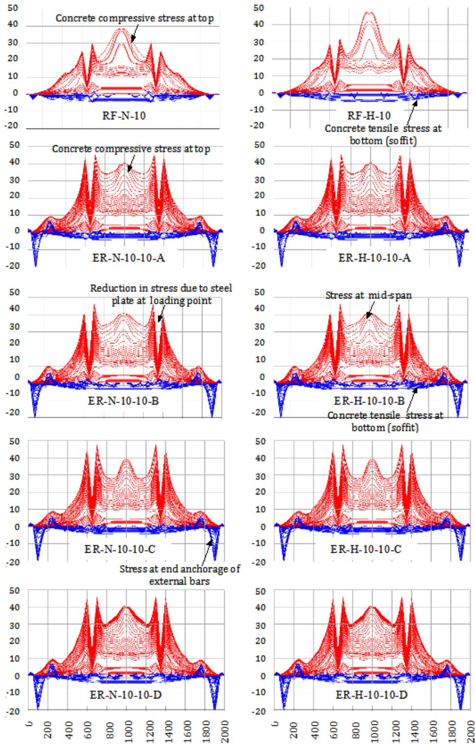
Fig. 5 Stress distribution in concrete top (compression) and bottom (tension) surfaces
