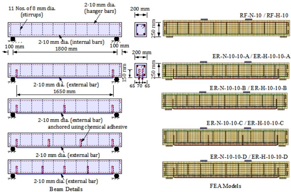
Fig. 1 Details of beam specimen and FEA Models
