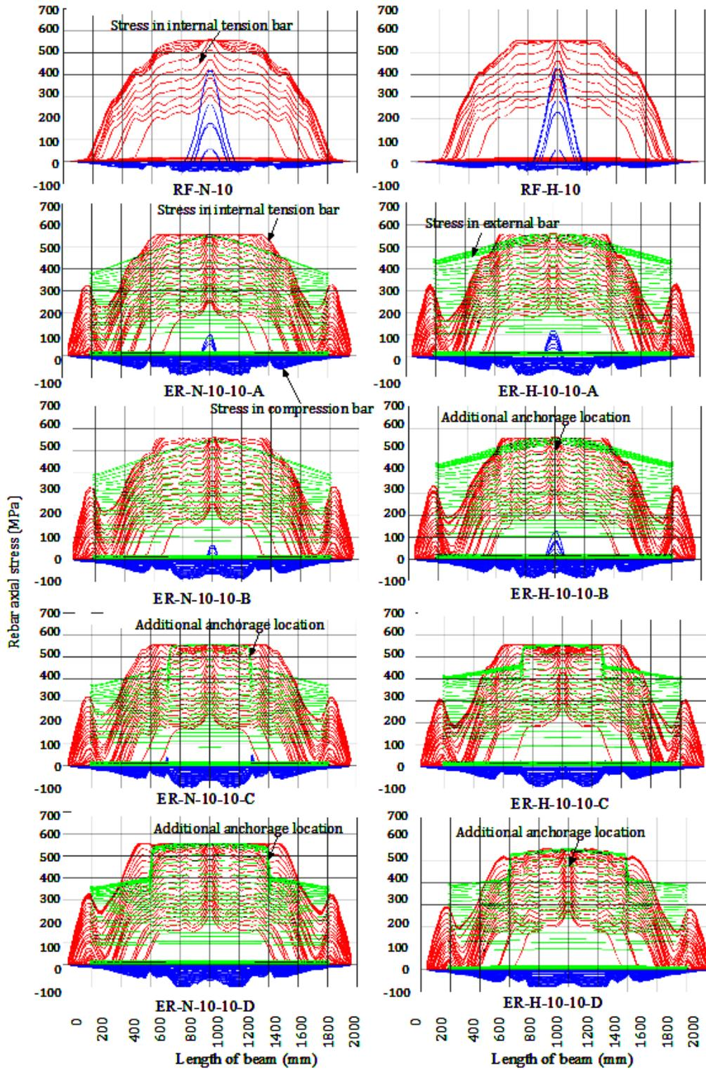
Fig. 6 Axial stress in internal, external and compression bars
