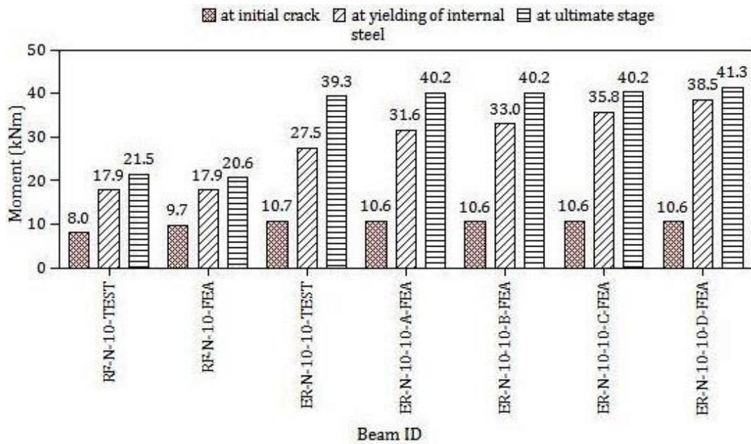
Fig. 7 Comparison of moment at critical stages– N-10 series
