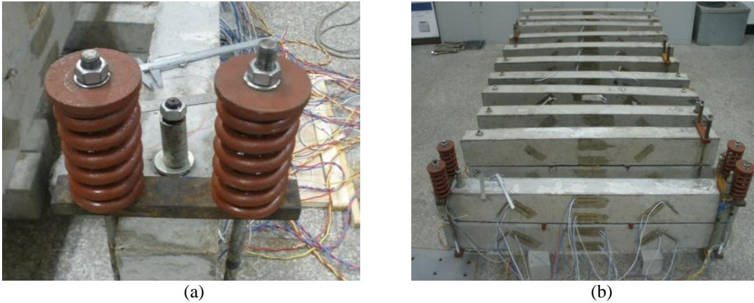
Fig. 3 (a) Loading application and (b) strain measurements Fu, Ye, et al. 2015
