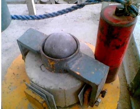
Fig. 1(a) Close-up view of the impact test set up
