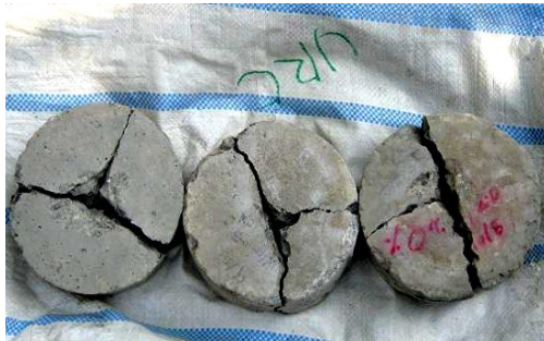
Fig. 2(a) Silica fume concrete (HPC) disc specimens after failure
