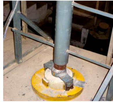
Fig. 1(b) Disc specimen under drop weight impact test
