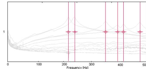
Fig. 12 The spectral density plot for each singular value of the damaged dam model
