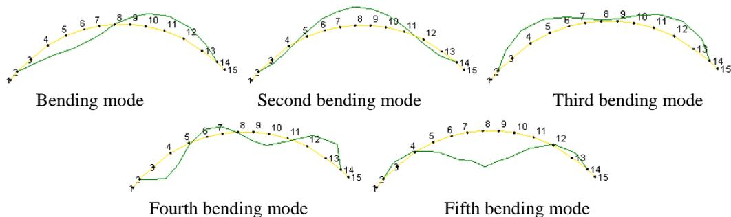
Fig. 13 The first five mode shapes of the dam for the damaged case
