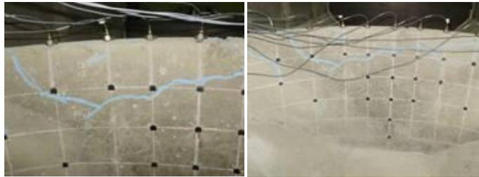
Fig. 11 The observed damage distribution on the dam model
