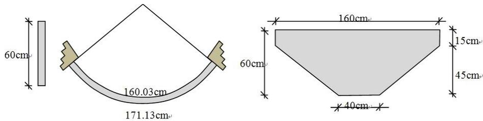
Fig. 1 The arch type dam model and its dimensions (Sevim, 2010)
