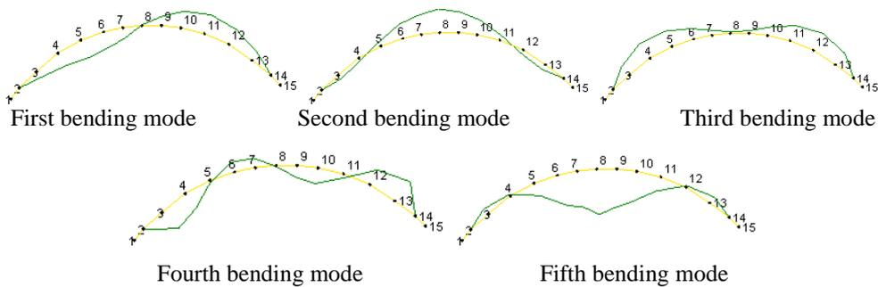
Fig. 9 The first five mode shapes of the dam for the undamaged case
