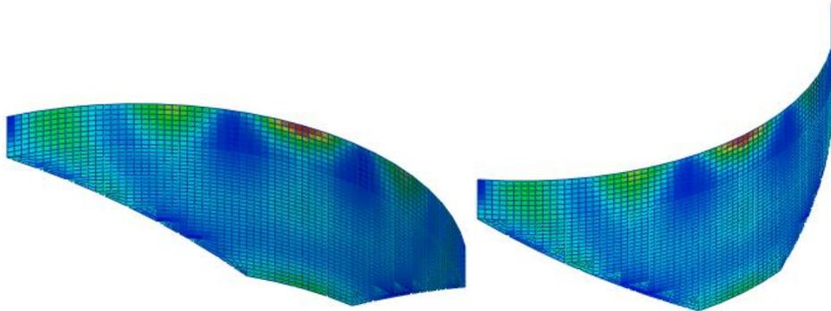
Fig. 10 The distribution of the elasticity modulus in the calibrated finite element model
