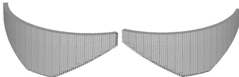
Fig. 2 The initial finite element model of the dam
