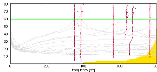
Fig. 7 The stability diagram for the undamaged case of the dam model
