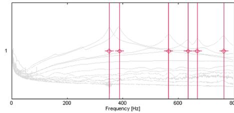
Fig. 8 The spectral density plots of each singular values for the undamaged dam model
