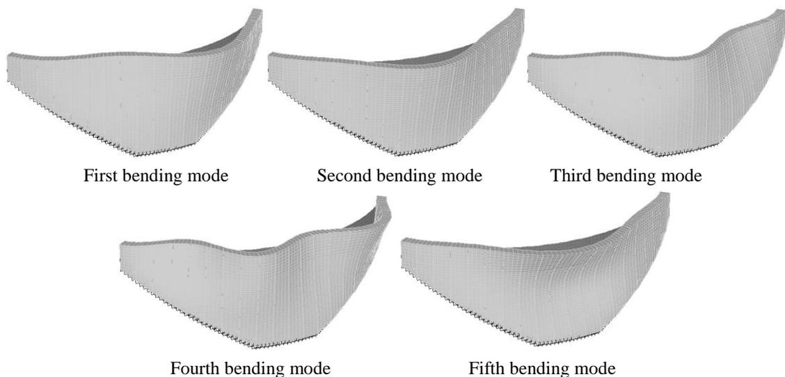
Fig. 3 The mode shapes of the dam model for initial case
