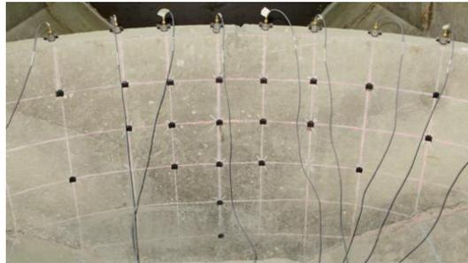
Fig. 5 A typical view from the accelerometer connection and direction on the dam model
