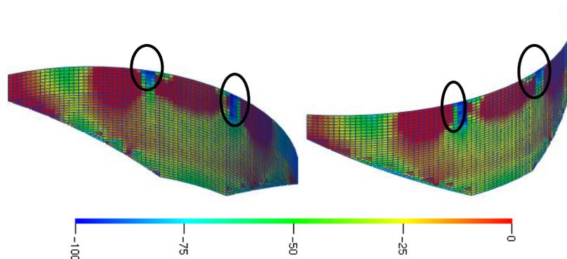
Fig. 14 The web thickness change after model updating on the dam body
