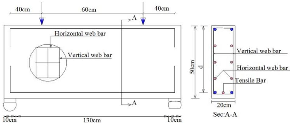
Fig. 1 Geometrical details of tested deep beams
