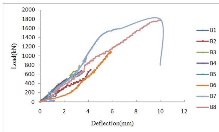
Fig. 6 Deflection of tested HSSCC deep beams at mid span
