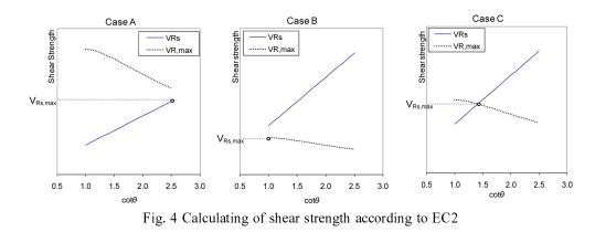
The model uncertainties of the shear capacity are taken into account by inserting a random variable  $(Y_{VR})$  into the shear strength model of EC2.  $Y_{VR}$  is supposed to be lognormal random variable with a mean value of 1 and coefficient of variation equal to 0.35 (Mwafy and Elnashai 2008). The shear strength is calculated as
