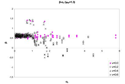
Fig. 7 Safety index  $\beta$  as a function of  $\alpha_c$  and v, for  $\gamma_{Rd} = 1.3$
