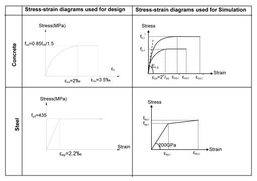
Fig. 3 Stress-strain diagrams of concrete and steel
