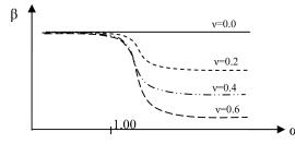
Fig. 9 Schematically presentation of  $\beta$  as a function of  $\nu$  and  $\alpha_c$ .  $\beta$  is also affected from  $\gamma_{Rd}$  and  $\cot\theta$ ,  $\beta$  takes larger values when  $\gamma_{Rd}$  increases and when  $\cot\theta$  decreases
