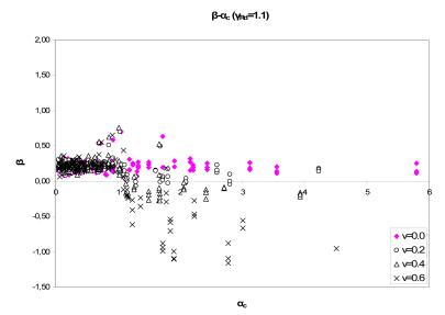
Fig. 6 Safety index  $\beta$  as a function of  $\alpha_c$  and  $\nu$ , for  $\gamma_{Rd} = 1.1$
