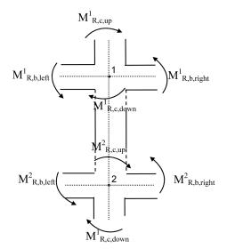
Fig. 1 Directions of the resisting moments for calculating relation 3
