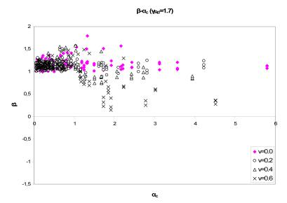
Fig. 8 Safety index  $\beta$  as a function of  $\alpha_c$  and v, for  $\gamma_{Rd} = 1.7$
