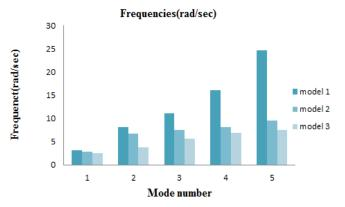
Fig. 4 Effect of reservoir and foundation on the modal frequencies of the dam
