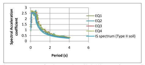
Fig. 5 Response spectra of accelerograms along with IS 1893 spectrum for Type II soil
