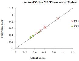
Fig. 2 Plot for first and second mode periods of dam (full reservoir)- comparison of empirical and modal analysis values
