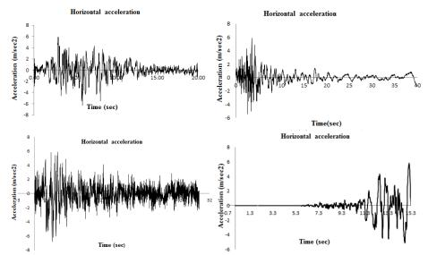
Fig. 6 Acceleration-time history of earthquake records made compatible with IS 1893 spectrum for Type II soil with a PGA of 0.6 g
