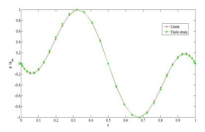
Fig. 6 Cross section rotation of the third mode of the clamp-clamp supported carbon/epoxy composite beam
