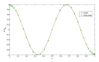
Fig. 15 Cross section rotation of the third mode of the simply-simply supported carbon/epoxy composite beam
