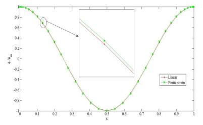
Fig. 14 Cross section rotation of the second mode of the simply-simply supported carbon/epoxy composite beam
