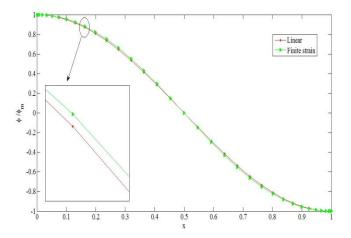
Fig. 13 Cross section rotation of the first mode of the simply-simply supported carbon/epoxy composite beam
