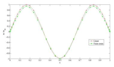
Fig. 12 Deflection of the third mode of the simply-simply supported carbon/epoxy composite beam
