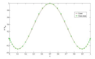
Fig. 5 Cross section rotation of the second mode of the clamp-clamp supported carbon/epoxy composite beam
