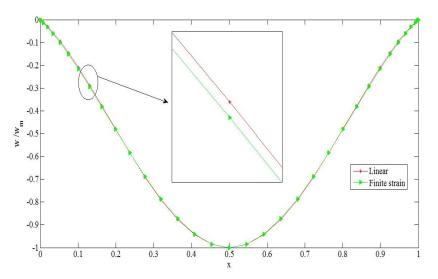
Fig. 1 Deflection of the first mode of the clamp-clamp supported carbon/epoxy composite beam
