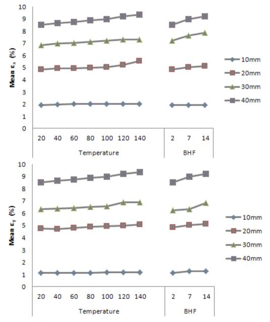
Fig. 9 Effects of strain on mean values of strain components at point 3 (Venkatesan 2012)
