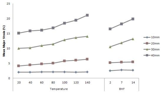
Fig. 8 Main effect of process parameters on mean major strain at point 3 (Venkatesan 2012)
