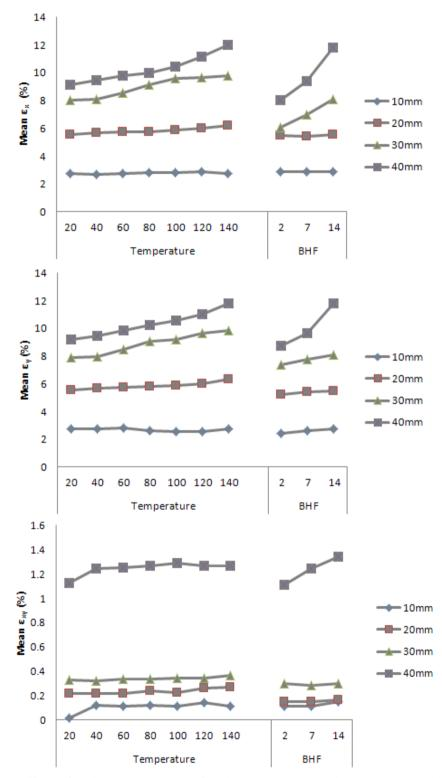
Fig. 5 Effects of strain on mean values of strain components at point 1(Venkatesan 2012)
