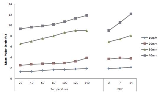
Fig. 6 Main effect of process parameters on mean major strain at point 2 (Venkatesan 2012)
