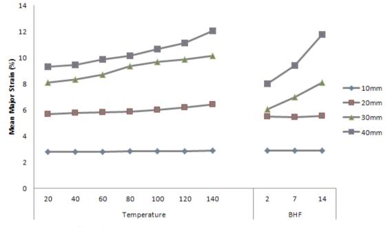
Fig. 4 Main effect of process parameters on mean major strain at point 1 (Venkatesan 2012)
