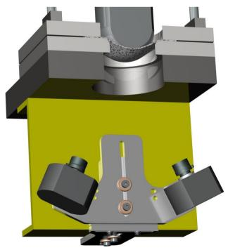
Fig. 1 Schematic representation of ARAMIS coupled with stamping press (Venkatesan 2012)
