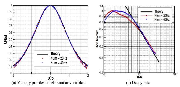
Fig. 5 Synthetic jet in a quiescent air: b(y) is the jet width at the selected y; h is the actuator slot width
