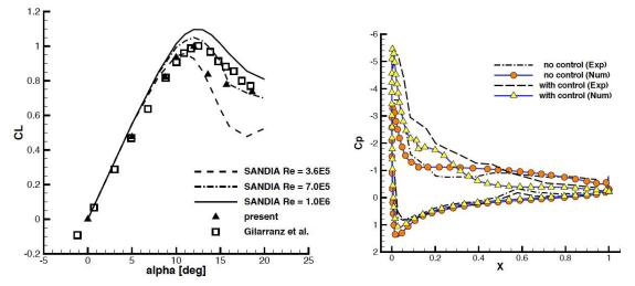
(a) Comparison of present numerical results against experimental data (Gilarranz *et al.* 2005, Sheidahl and Klimes 1981) of the baseline lift coefficient
