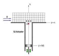
Fig. 1 A sketch of synthetic jet actuator model and its coupling with the main flow domain
