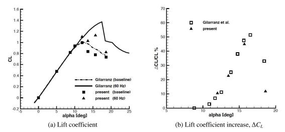
Fig. 11 Active control of NACA0015 airfoil. Comparison of present numerical results with the experimental data of (Gilarranz *et al.* 2005) at 60Hz
