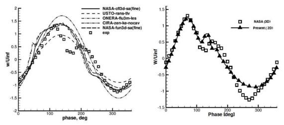
(a) Vertical velocity at the SJ orifice center for test-case 2 as reported in Rumsey *et al.* (2006)
