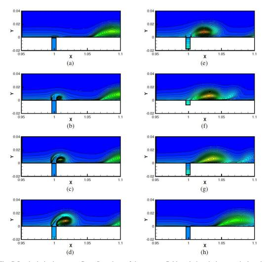
Fig. 7 Synthetic jet in a cross-flow. Snapshots of the entropy field evolution during a typical cycle of flow forcing by synthetic jets actuation
