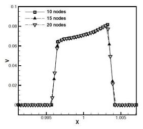
Fig. 8 Instantaneous velocity profile at the actuator exit. The curves refer to the number of nodes (10, 15 and 20) used to resolve the SJ velocity profile, for grids with  $180 \times 90$ ,  $240 \times 120$ ,  $320 \times 150$  nodes, respectively
