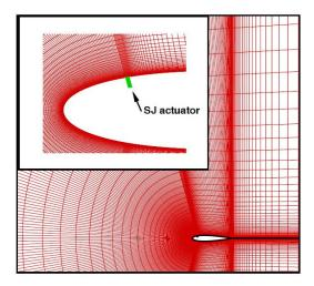
Fig. 9 A sketch of 507×121 the stretched grid around NACA0015 airfoil and on the SJ actuator
