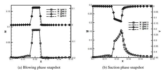
Fig. 13 NACA0015 test-case. Instantaneous profiles of Mach number and wall-normal velocity on the airfoil region close to SJ actuator orifice. Grid1 (507x121) and grid2 (518x121) have 10 and 20 nodes along the actuator slot width, respectively.
