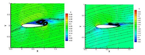
(a) Unmanipulated, stalled flow field
