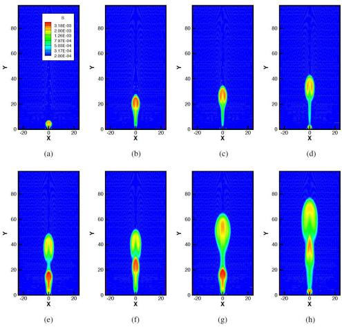
Fig. 4 Synthetic jet in quiescent air. The generation of the vortex flow and its evolution time for the case with  $f_2$ =40 Hz. Snapshots sequence of the entropy field at different time steps. Entropy is related to vorticity through Crocco's equation. Times scaled to the period *T* are: (a) *t*=0.25T; (b) *t*=0.63T; (c) *t*=0.83T; (d) *t*=1.17T; (e) *t*=1.46T; (f) *t*=1.67T; (g) *t*=2.5T; (h) *t*=3.2T
