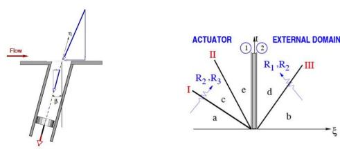
(a) Sketch of SJ configuration (b) Wave propagation pattern at the actuator orifice Fig. 3 SJ actuator during suction
