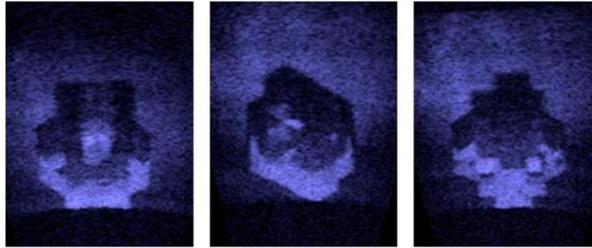
Fig. 1 Appearance of the same object in sonar images changing depending on the viewing angles
