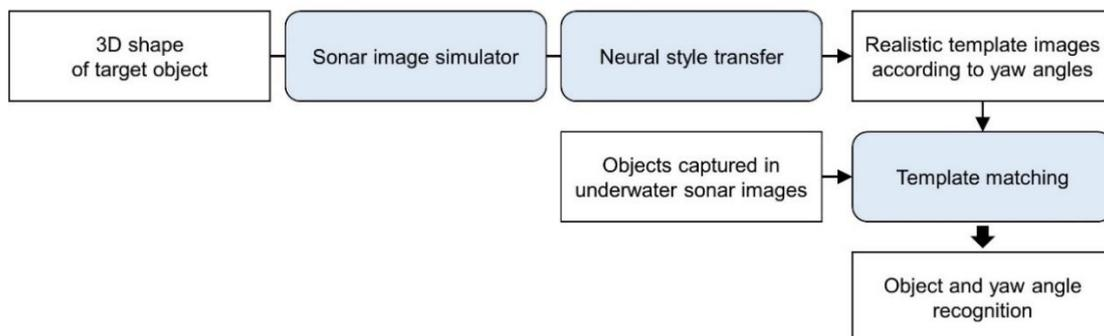
Fig. 2 The proposed method for underwater objects' yaw estimation
