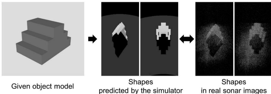
Fig. 5 Difference between the simulated shapes and real sonar images of an object
