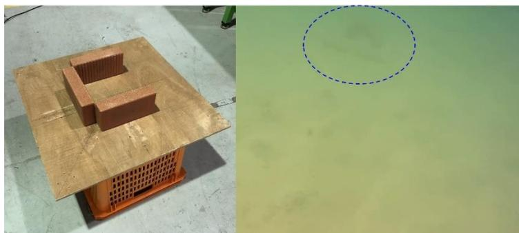
Fig. 12 Designed landmark for the bearing estimation of the AUV in the sea trials
