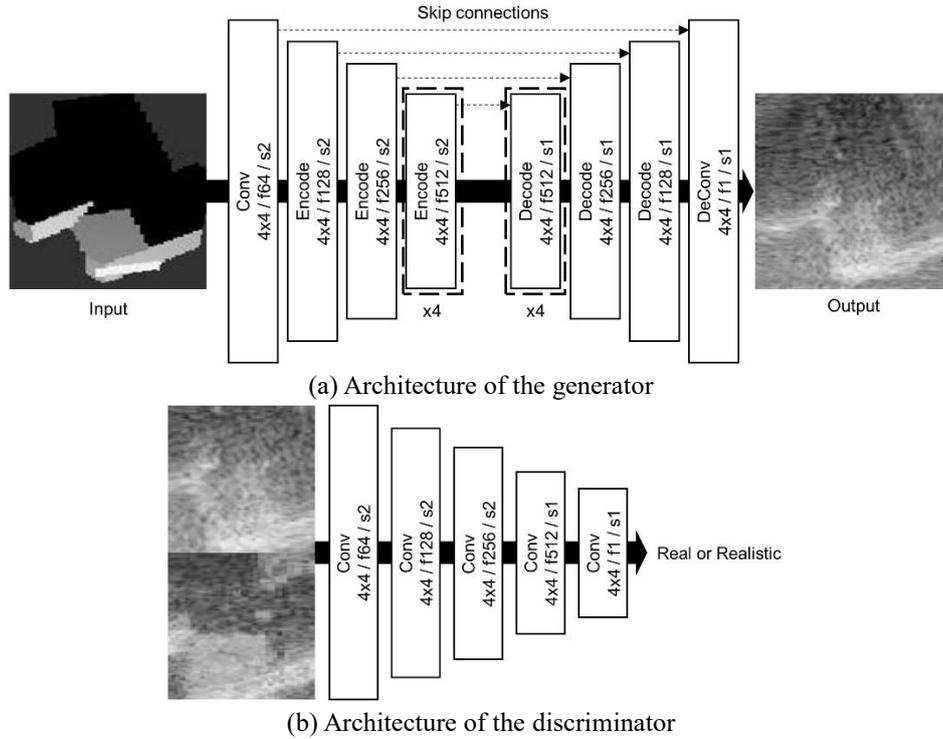
Fig. 6 Architecture of the neural network for simulating the realistic sonar images. 4x4 is the size of the convolutional kernel, f denotes the kernel depth, and s means the stride of the kernel
