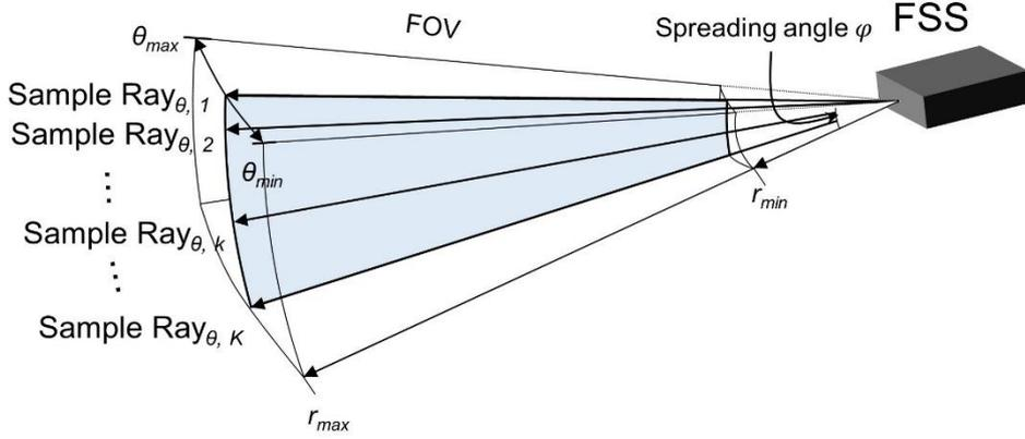
Fig. 4 Acoustic beam modeling and terminologies for the FSS simulator
