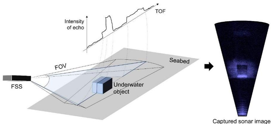
Fig. 3 Imaging mechanism of the FSS
