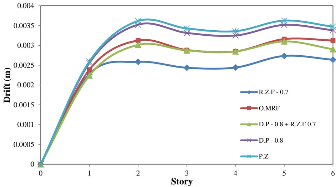
Fig. 6 Drift results of 6 story frame (R.Z.F. = 0.7, D.P. = 0.8)
