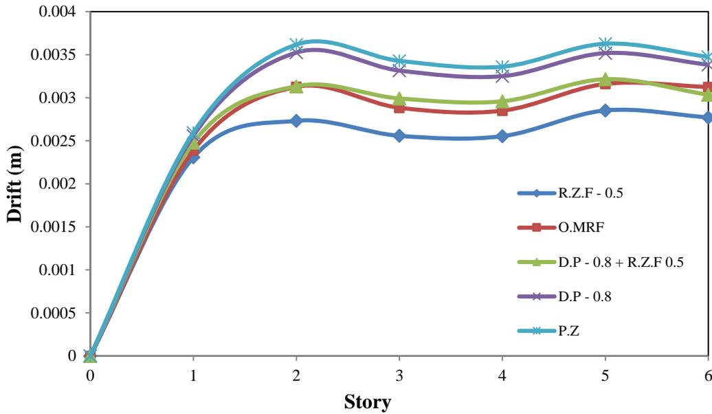
Fig. 5 Drift results of 6 story frame (R.Z.F. = 0.5, D.P. = 0.8)
