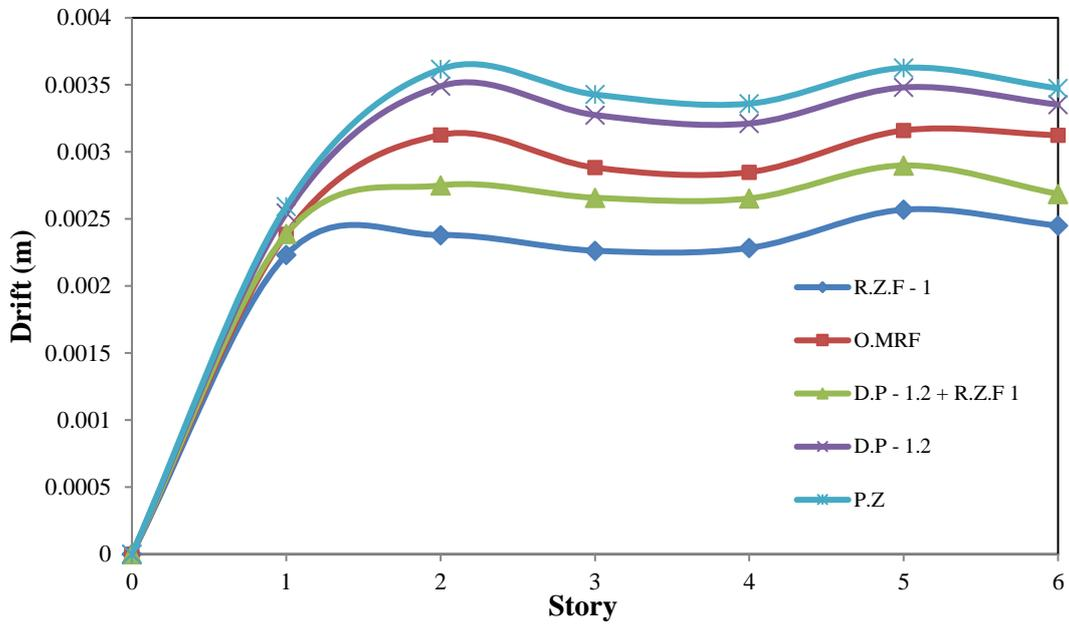
Fig. 12 Drift results of 6 story frame (R.Z.F. = 1.0, D.P. = 1.2)
