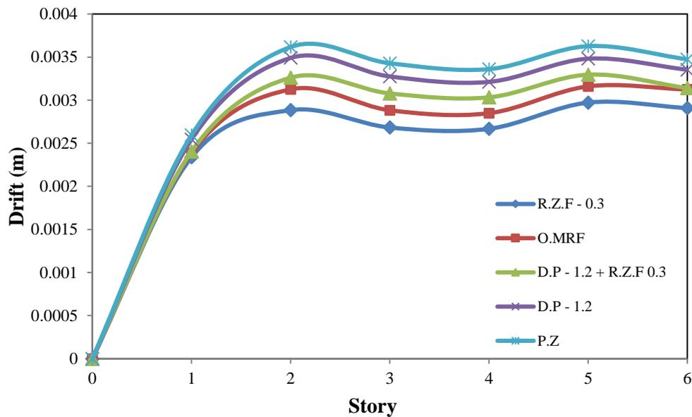
Fig. 9 Drift results of 6 story frame (R.Z.F. = 0.3, D.P. = 1.2)
