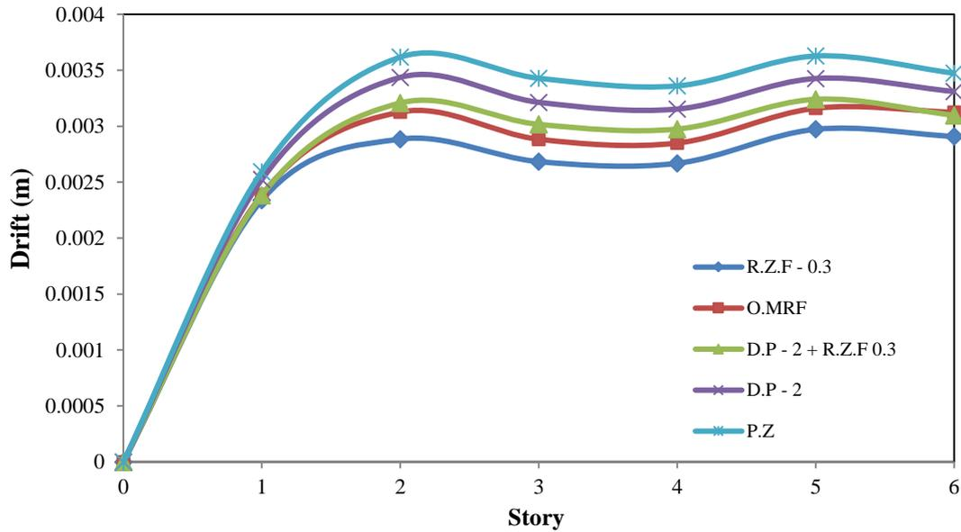
Fig. 14 Drift results of 6 story frame (R.Z.F. = 0.3, D.P. = 2.0)
