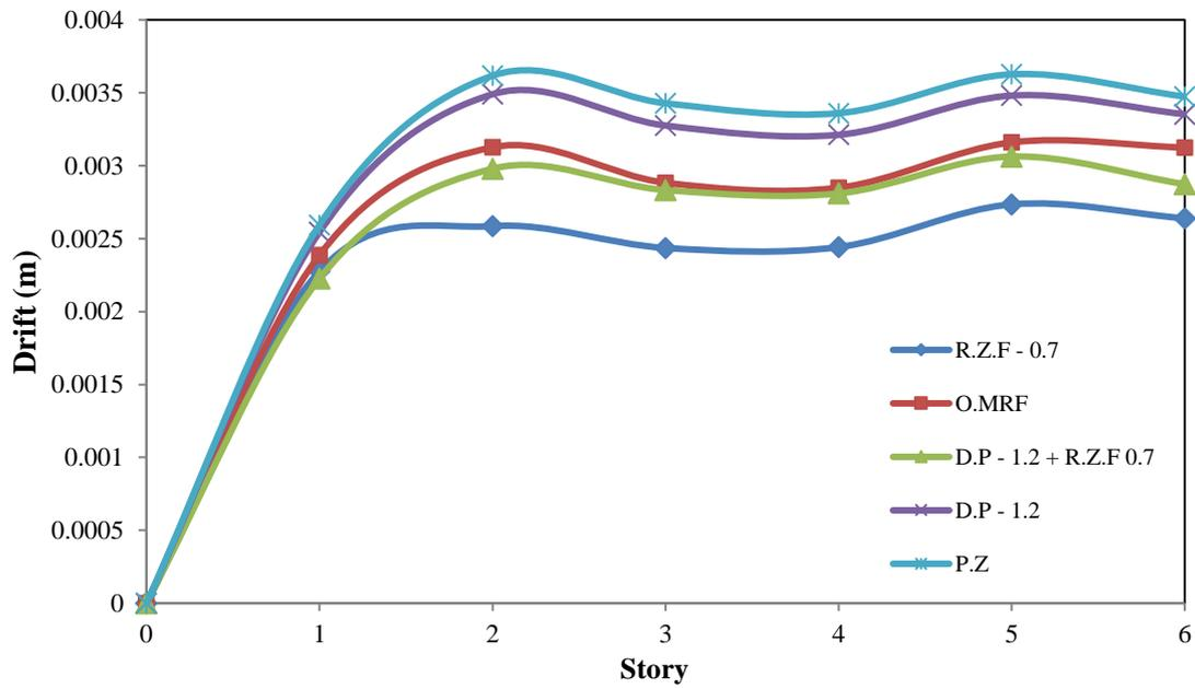
Fig. 11 Drift results of 6 story frame (R.Z.F. = 0.7, D.P. = 1.2)
