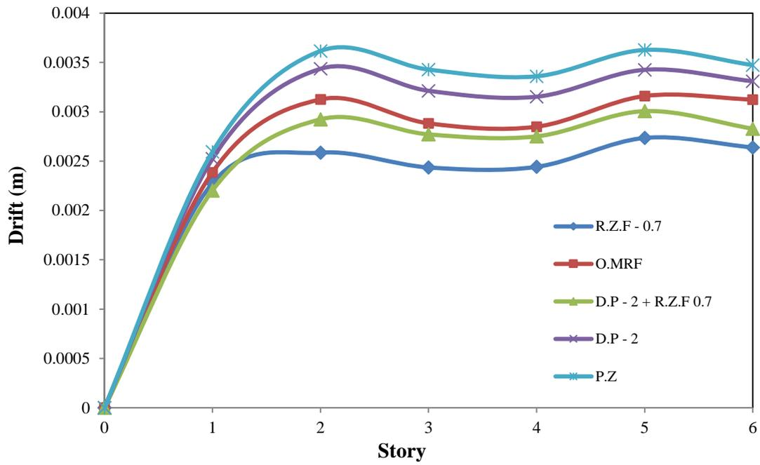
Fig. 16 Drift results of 6 story frame (R.Z.F. = 0.7, D.P. = 2.0)
