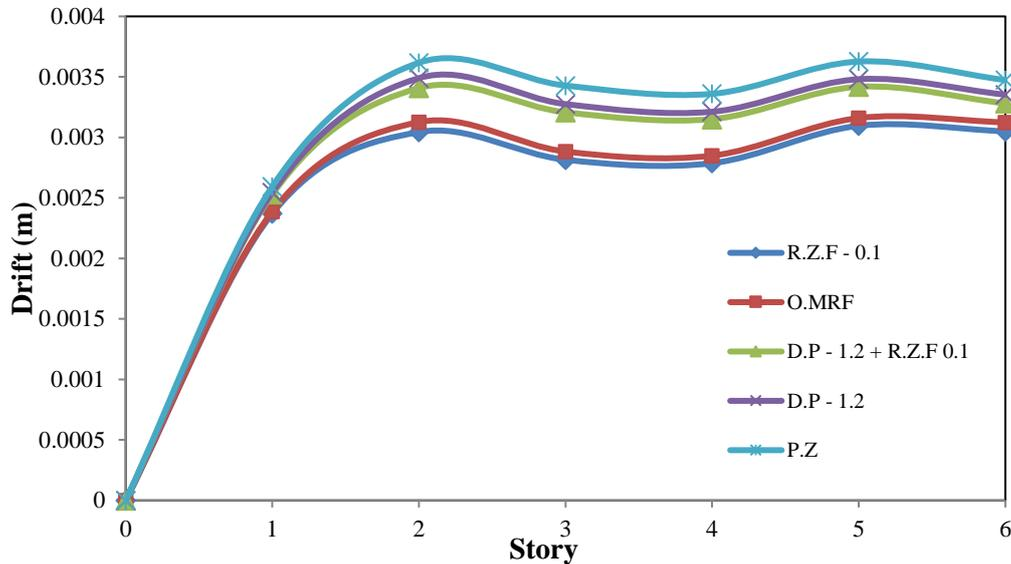
Fig. 8 Drift results of 6 story frame (R.Z.F. = 0.1, D.P. = 1.2)
