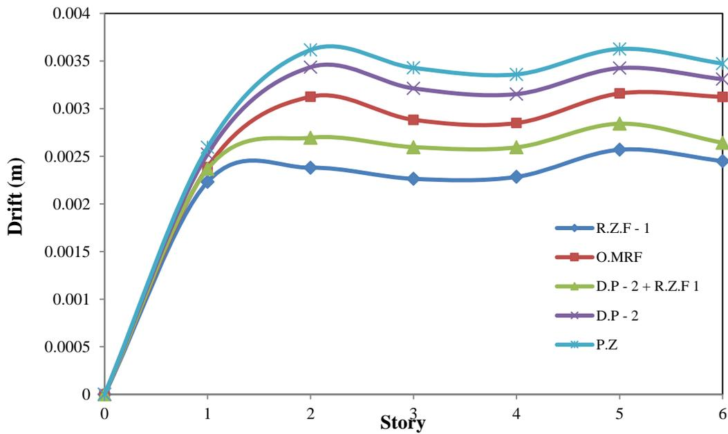
Fig. 17 Drift results of 6 story frame (R.Z.F. = 1.0, D.P. = 2.0)
