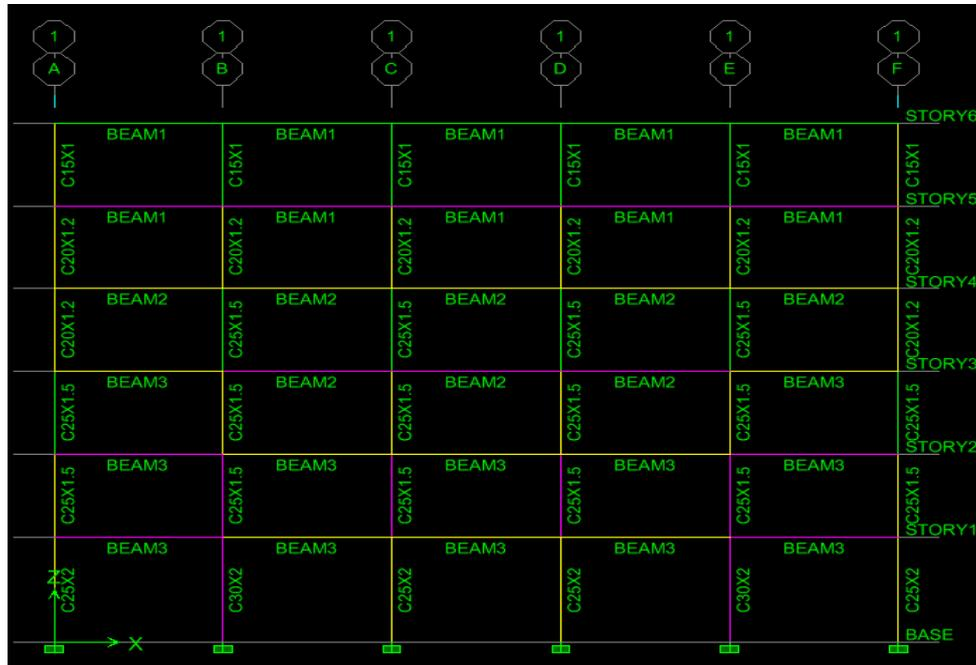
Fig. 2 Typical beams and columns in 6 stories frames
