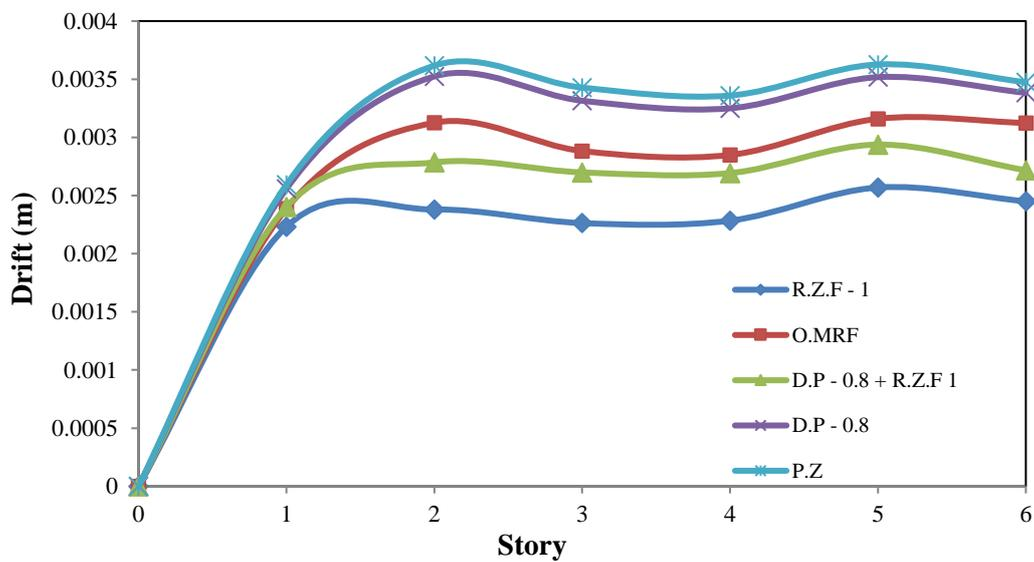
Fig. 7 Drift results of 6 story frame (R.Z.F. = 1.0, D.P. = 0.8)
