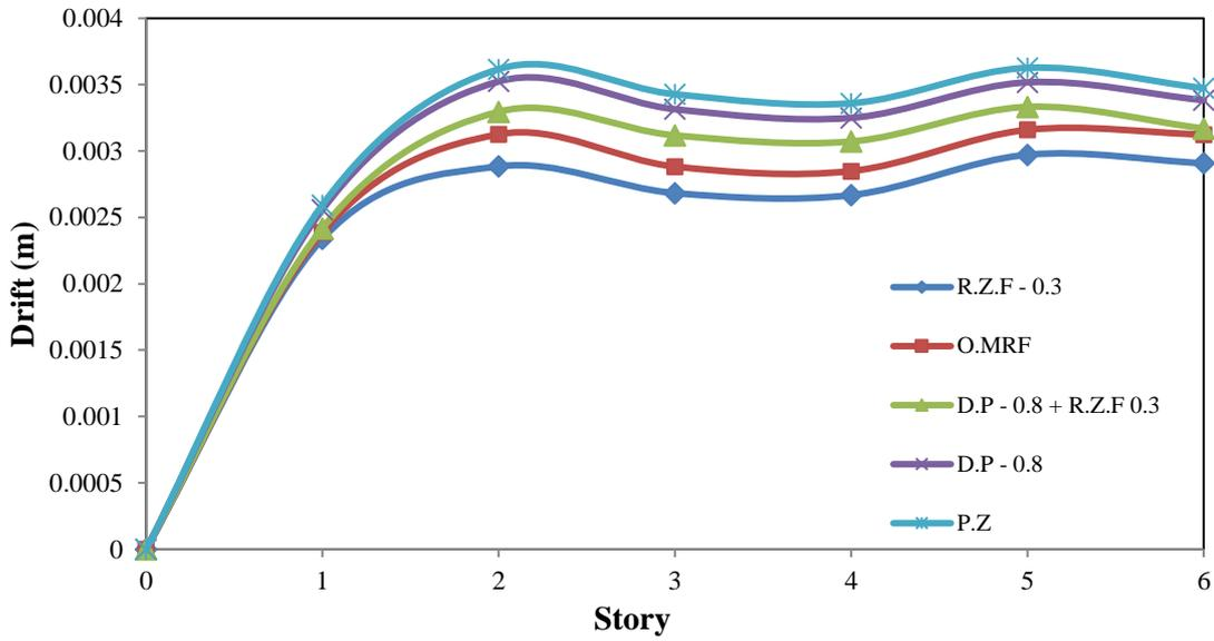
Fig. 4 Drift results of 6 story frame (R.Z.F. = 0.3, D.P. = 0.8)
