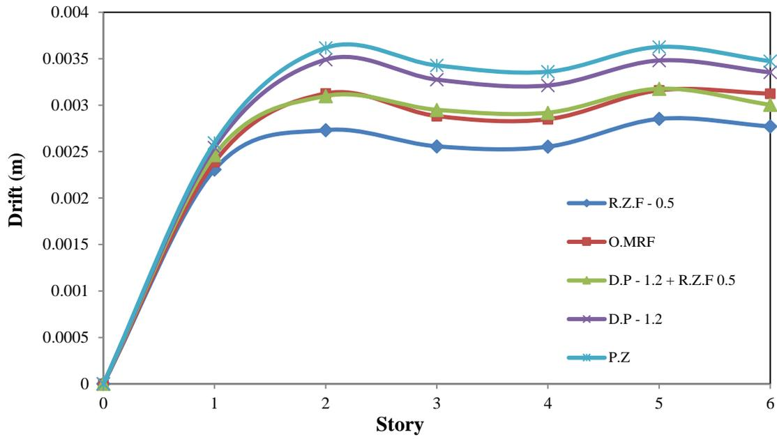
Fig. 10 Drift results of 6 story frame (R.Z.F. = 0.5, D.P. = 1.2)
