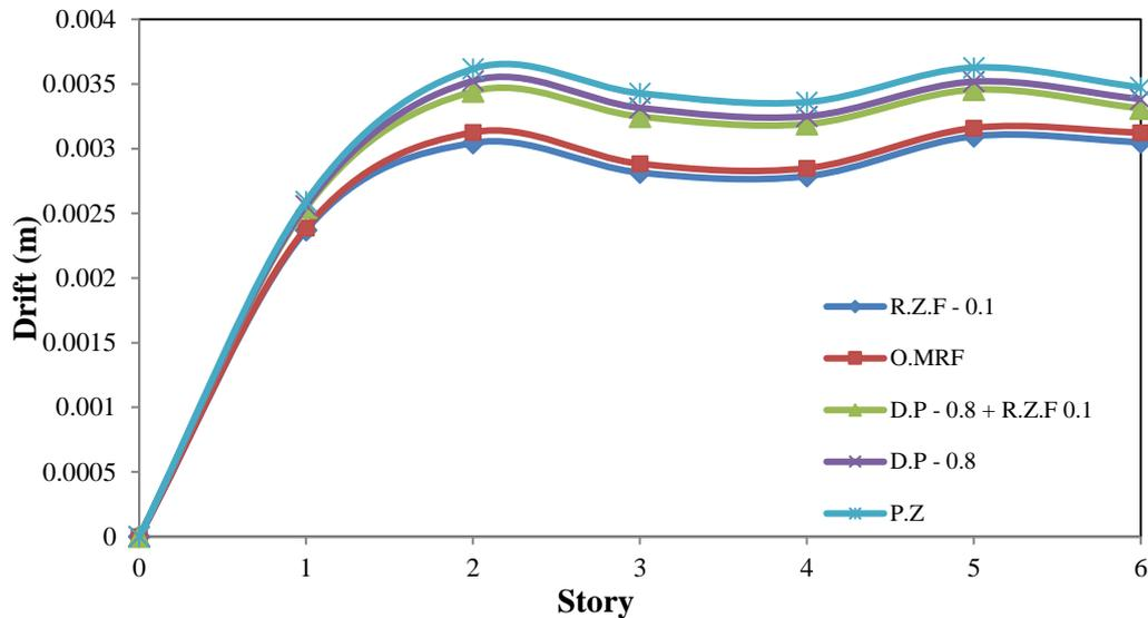
Fig. 3 Drift results of 6 story frame (R.Z.F. = 0.1, D.P. = 0.8)
