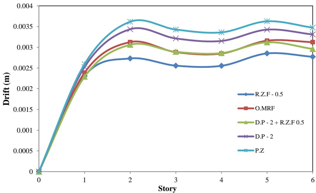
Fig. 15 Drift results of 6 story frame (R.Z.F. = 0.5, D.P. = 2.0)
